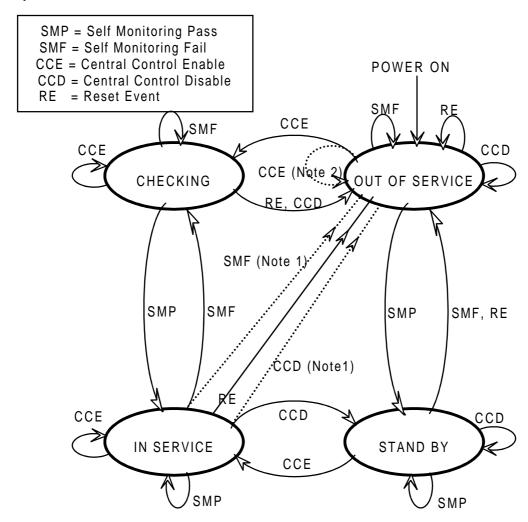
NOTE 1: In the "in-service" state, the occurrence of a SMF and/or CCD may result in a transition to the "out-of-service" state.
