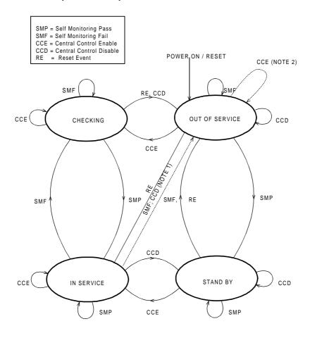
NOTE 1: In the "In Service" state, the occurrence of SMF and/or CCD may result in a transition to the "Out of Service" state.
