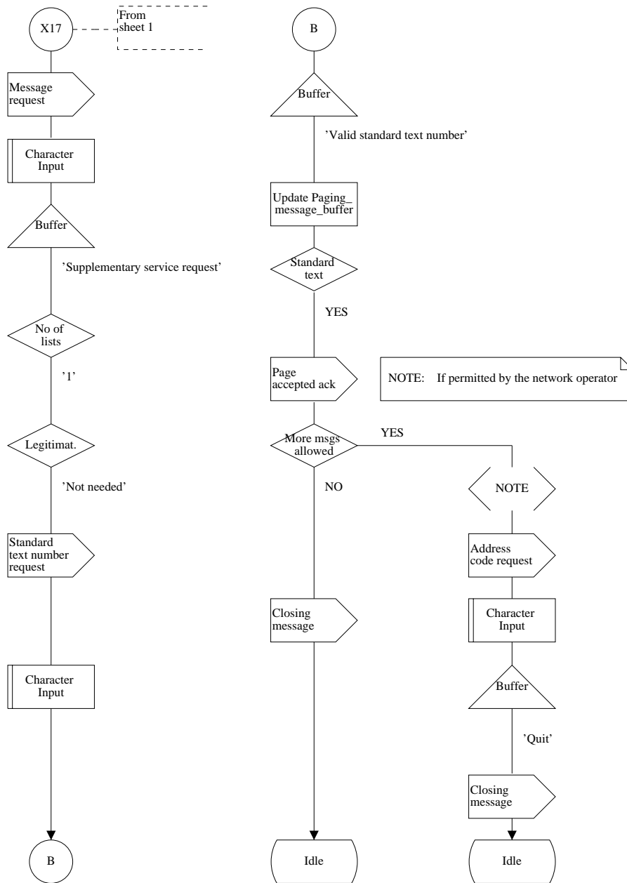
Figure G.1.2 (sheet 2 of 2): A typical two-stage selection call with level 1 priority and standard text
