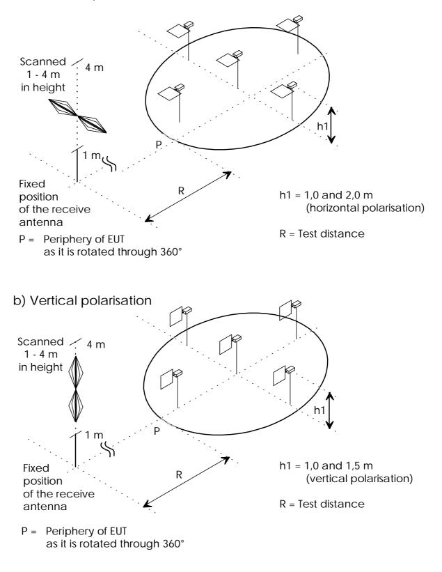
NOTE: The centre of the reference radiators align with the periphery of the test volume with the exception of the centre radiator.
