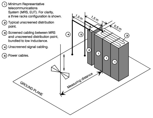
NOTE: Antenna scanned in height between 1 and 4 metres for horizontal and vertical polarisation.
