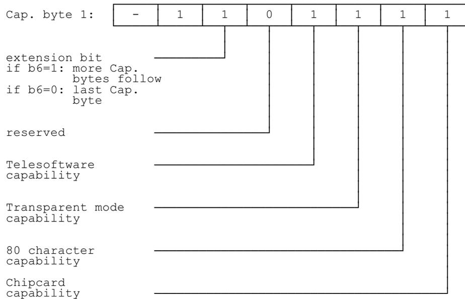
The Telesoftware capability bit and the Transparent mode capability bit shall be used to identify the use of these data types associated with the profiles. Subclause 6.2 gives codes that are used to identify SRM conformance to ETS 300 074 [6] (Transparent data) and ETS 300 075 [7] (Processable data).
