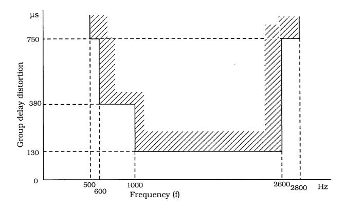
Figure 5: Group delay distortion limits with frequency
