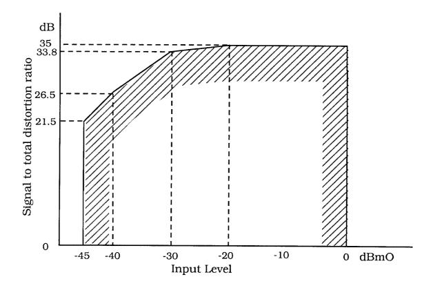
NOTE: The values of figure 11 include the limits for the coding process given in CCITT Recommendation G.714, figure 5 and the allowance for the noise contributed via signalling circuits from the PABX power supply and other analogue sources which is limited to -(67+3) dBm0p = -70 dBm0p for one 4-wire analogue interface by CCITT Recommendation G.123, § 3.
