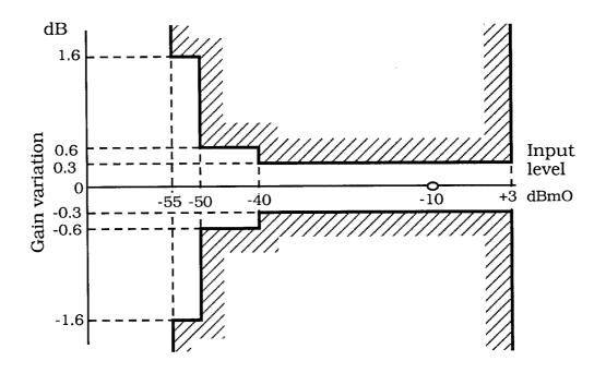
Figure 3: Variation of gain with input level
