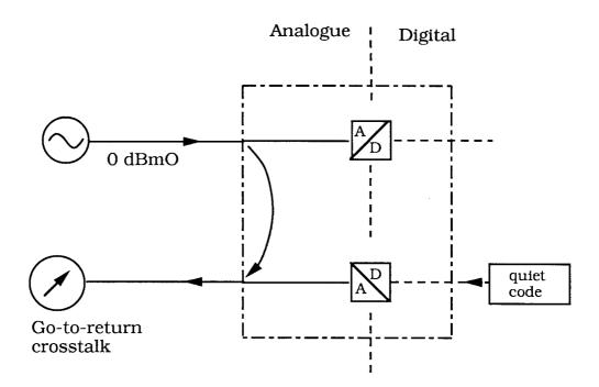
Figure 7: Measurement with an analogue test signal between go and return directions of the same half connection
