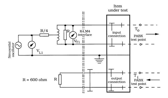
Longitudinal Conversion Loss (LCL) =  $20 \ 20 \ \log_{10} \left| \frac{V_{L1}}{V_{T1}} \right| dB$
