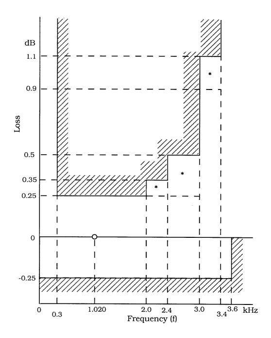
In the marked frequency ranges relaxed limits are shown which apply if the maximum length of cabling between cabinet and MDF (I-ETS 300 003, subclause 4.6) is used. The more stringent limits shown apply if no such cabling is present.
