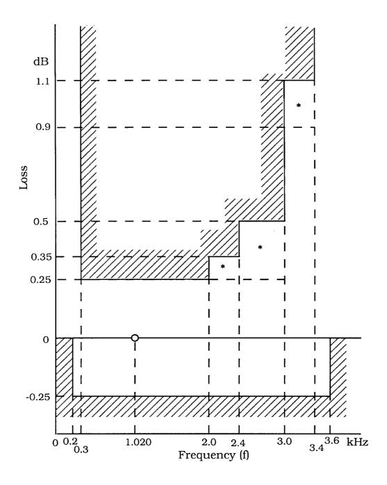
In the marked frequency ranges relaxed limits are shown which apply if the maximum length of cabling between cabinet and Main Distribution Frame (MDF) (I-ETS 300 003, subclause 4.6) is used. The more stringent limits shown apply if no such cabling is present.
