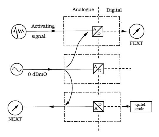
Figure 6: Measurement with an analogue test signal between different input connections of half connections
