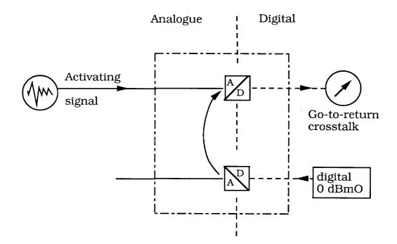
Figure 9: Measurement with a digital test signal between go and return directions of the same half connection
