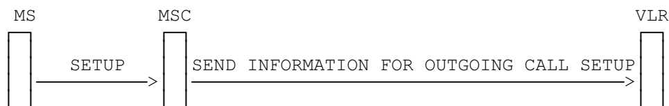
Figure 5.8: Signalling at explicit invocation of a CUG call
