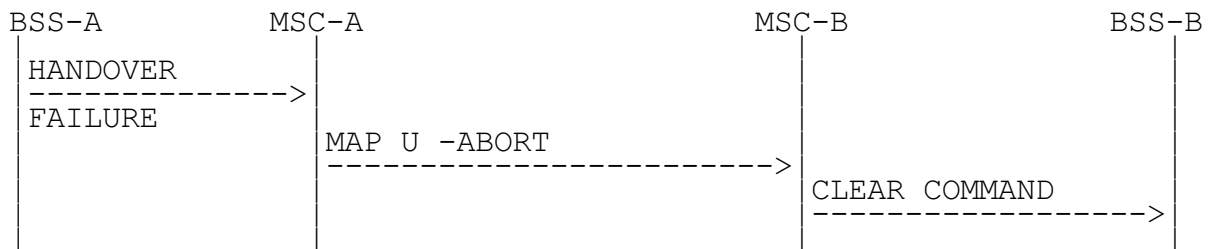
Figure 7: Signalling for Basic Inter-MSC Handover execution (Negative outcomes)
