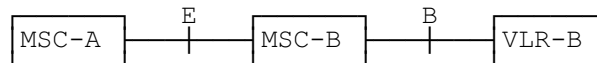
a) Basic handover procedure MSC-A to MSC-B and subsequent handover procedure MSC-B to MSC-A.
