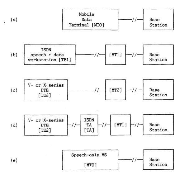
Figure 2/GSM 04.02: Examples of physical implementations
