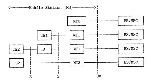
Figure 1/GSM 04.02 : GSM PLMN Access Reference Configuration
