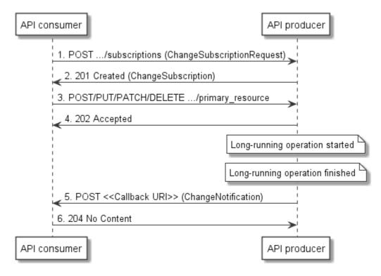
Figure 5.11.1-2: Asynchronous operation flow - with subscribe/notify
