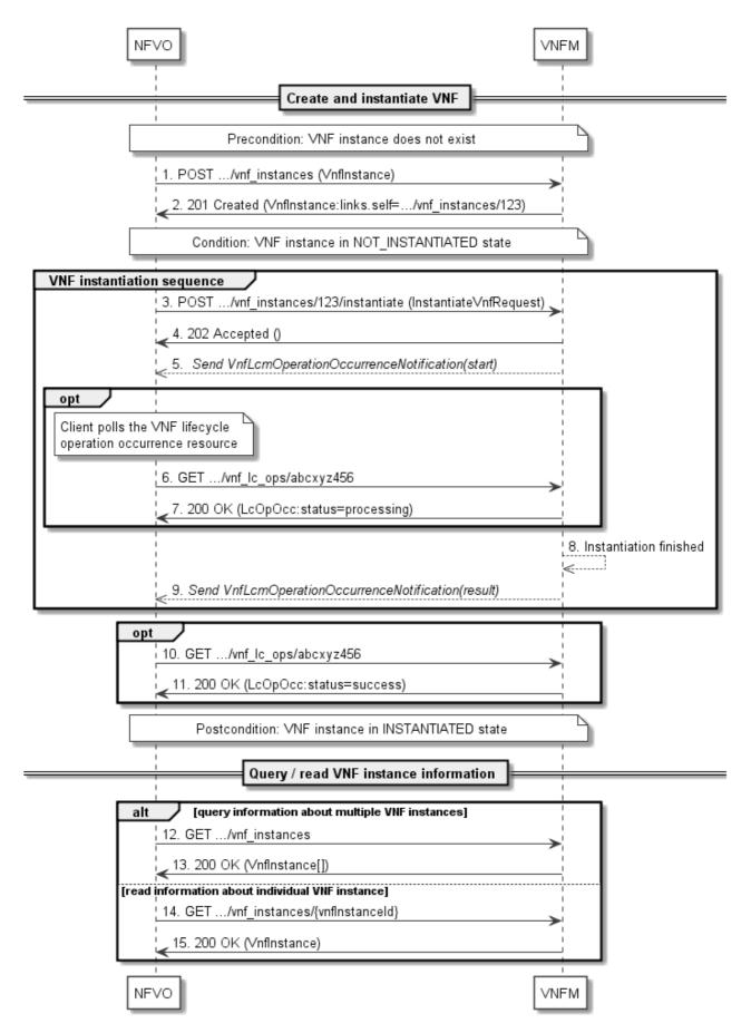
Figure B.2-2: Flow diagram resulting from the PlantUML source in figure B.2-1
