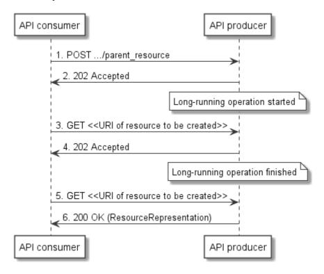
Figure 5.12.1-1: Asynchronous resource creation flow without monitor
