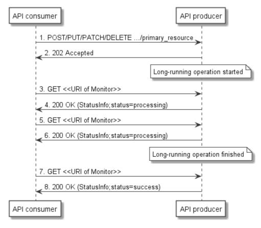
Figure 5.11.1-1: Asynchronous operation flow - with polling
