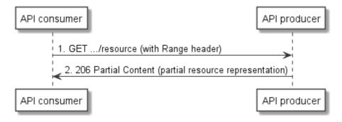
Figure 5.13.1-1: Flow of obtaining a partial representation of a resource
