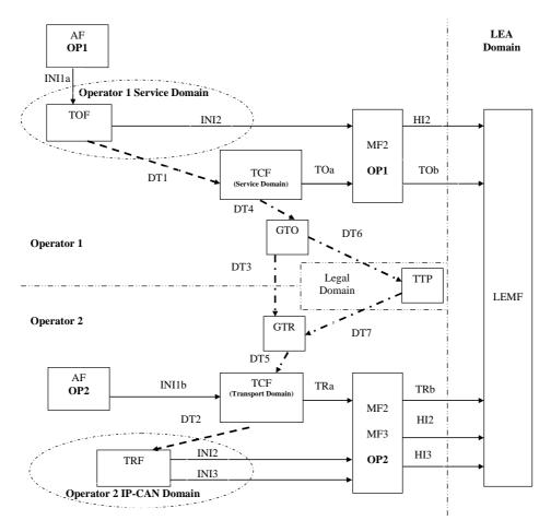
Figure A.2: Dynamic Triggering Multiple Operator Reference Model [i.5]
