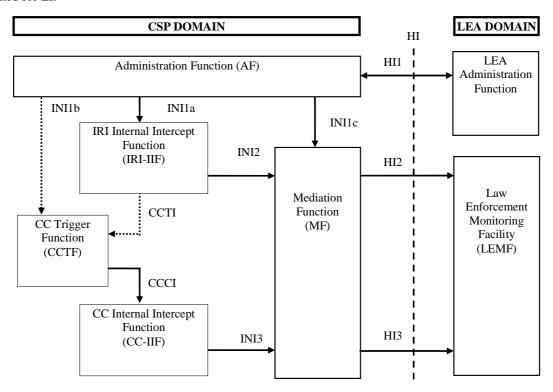
Figure A.1: Reference Model for IP Network LI from ETSI TR 102 528 [i.3]
