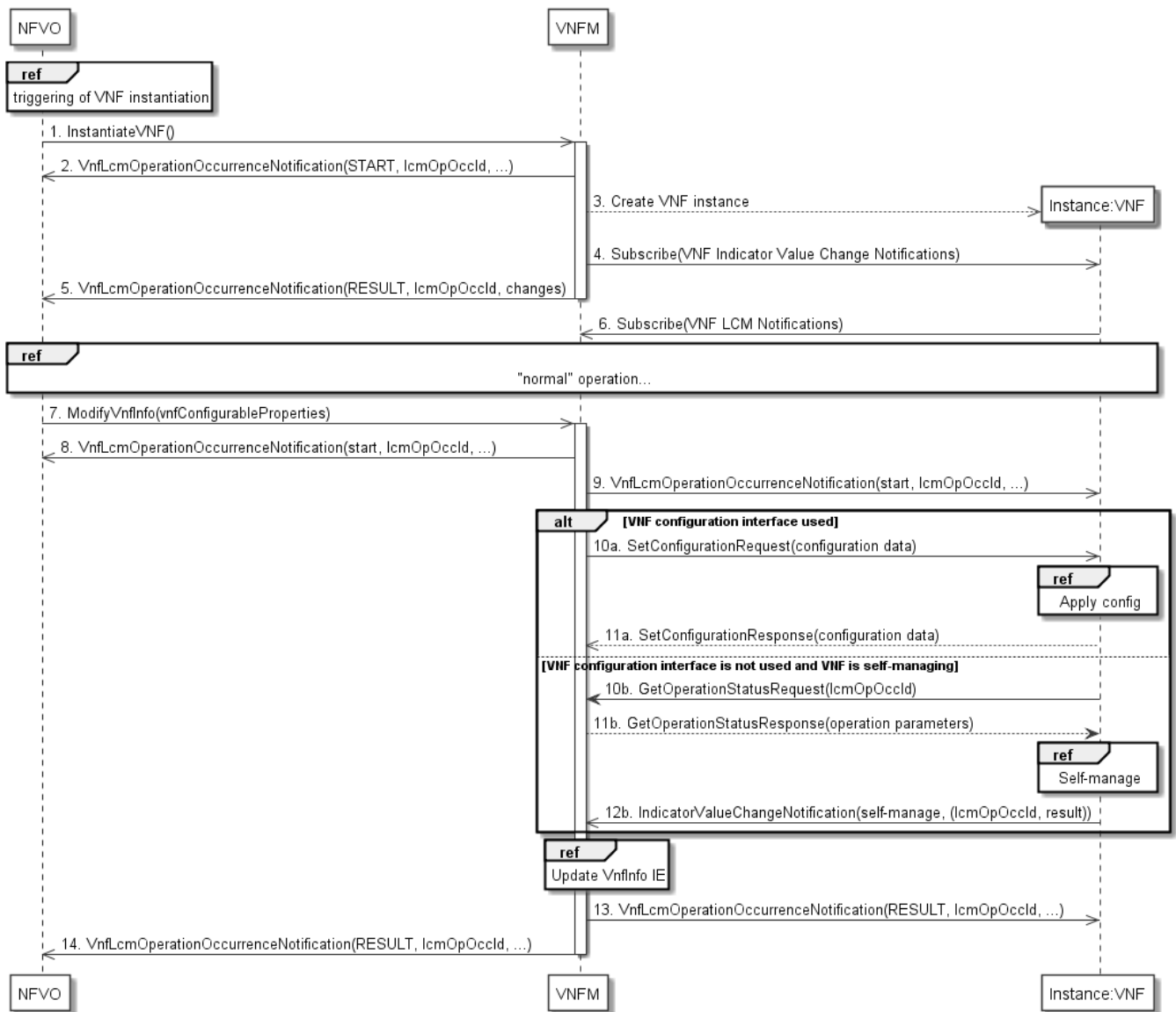
Figure B.1-1: Explicit change of VNF Configurable Properties
