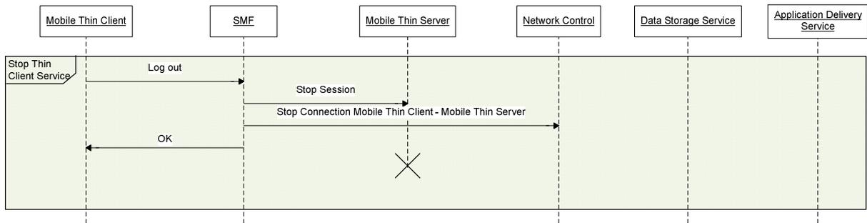
Figure A.4: Sequence diagram "Stop thin client service"
