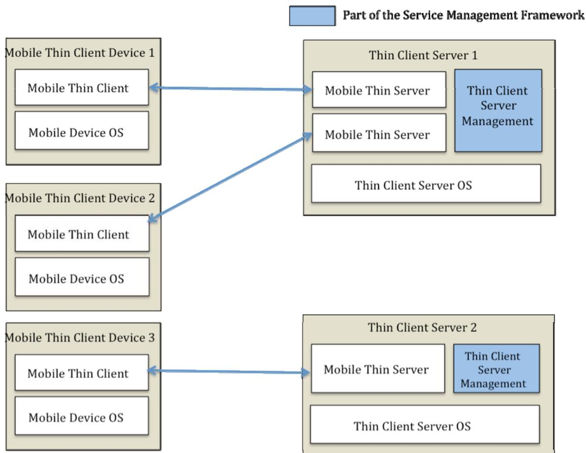
**Figure 2: Multi-user aspect of the system Architecture**
