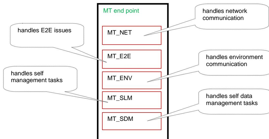
**Figure 10: System endpoint components**
