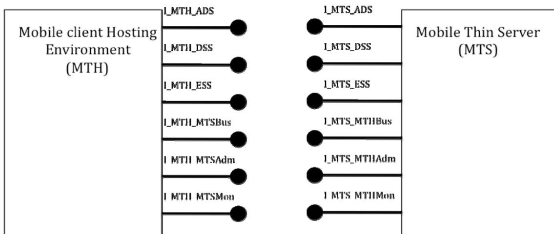
**Figure 13: Mobile Thin Server and its hosting environment interfaces (detailed)**
