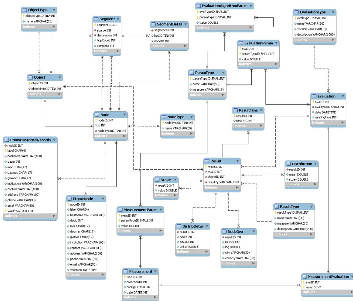
Figure 7: Schema used to store ETOMIC@ELTE active measurement data (B)
