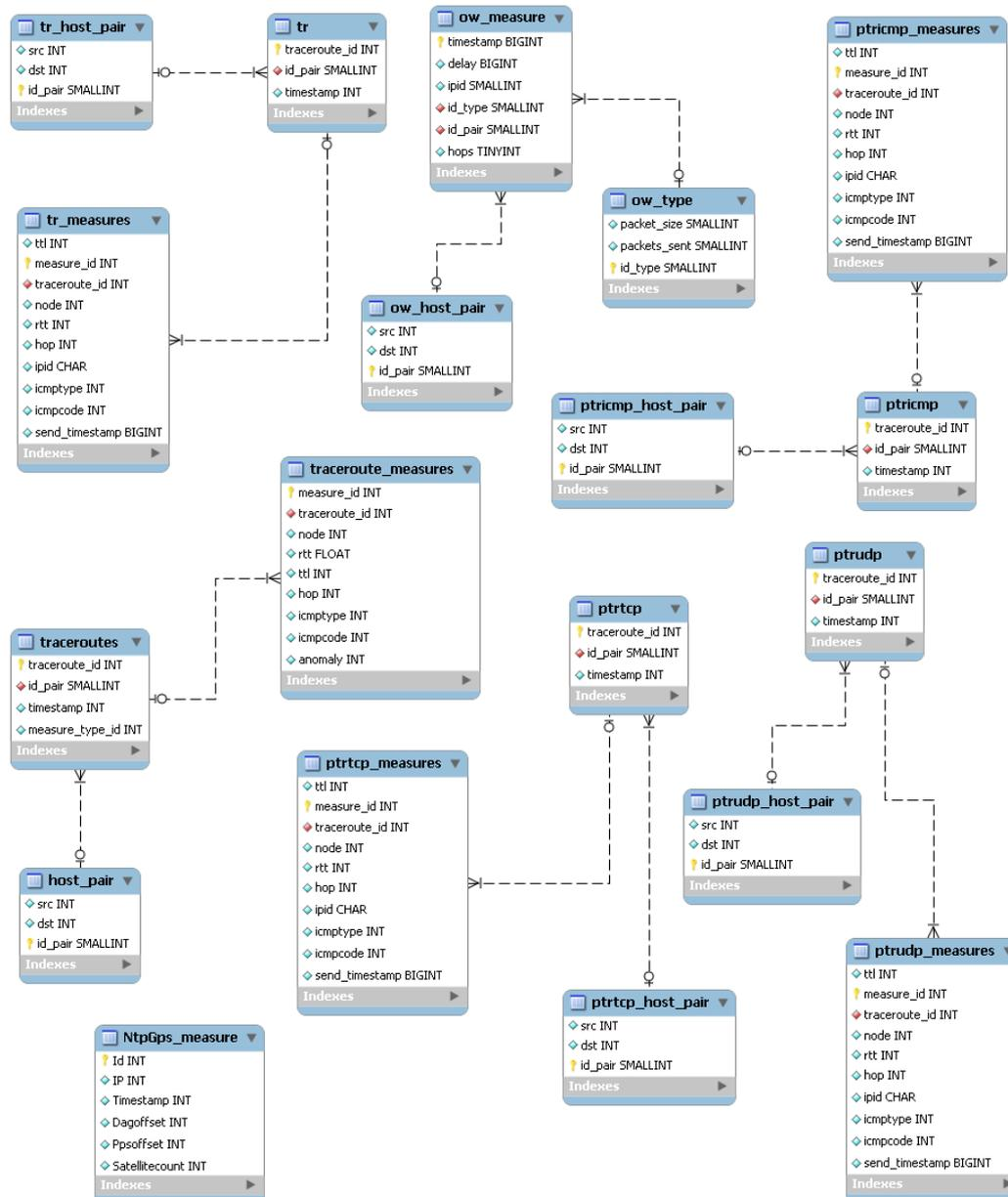
Figure 5: Schema used to store ETOMIC@UPNA pre-defined active measurement data
