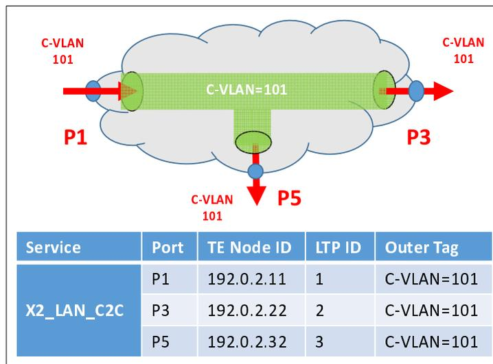
NOTE: Since all ports of the service require only Customer Bridge capabilities, the network can support only Customer Bridge functionality, Provide Bridge capabilities are not mandatory.
