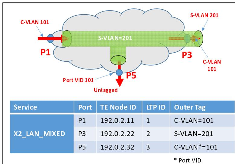
NOTE: Since P3 requires Provider Bridge capability, the network shall support Provider Bridging for the whole service.
