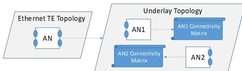
**Figure D.1.2.1: AL1 Ethernet Topology: Partial Connectivity, VLAN Transparency**
