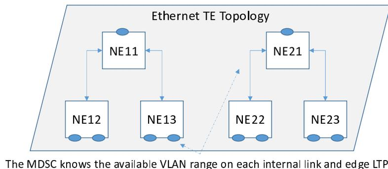
**Figure 4.3.3.2.2.1: AL2 Ethernet Topology: Partial Connectivity, VLAN Transparency**
