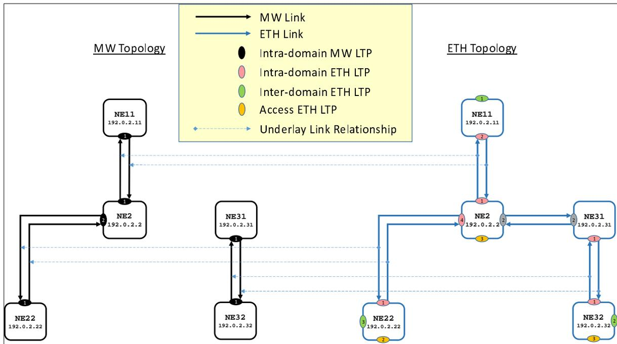
NOTE: The `ltp-id` values are local to the node, in this example they are (arbitrarily) numbered from 1 upwards, independently.
