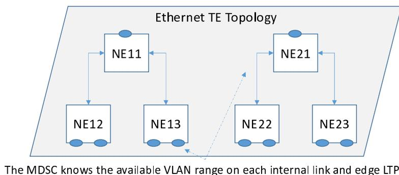
**Figure 4.3.3.2.2.1: AL2 Ethernet Topology: Partial Connectivity, VLAN Transparency**
