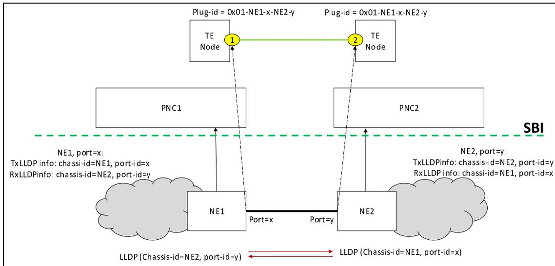
Figure B.2.1: Algorithm Block Diagram
