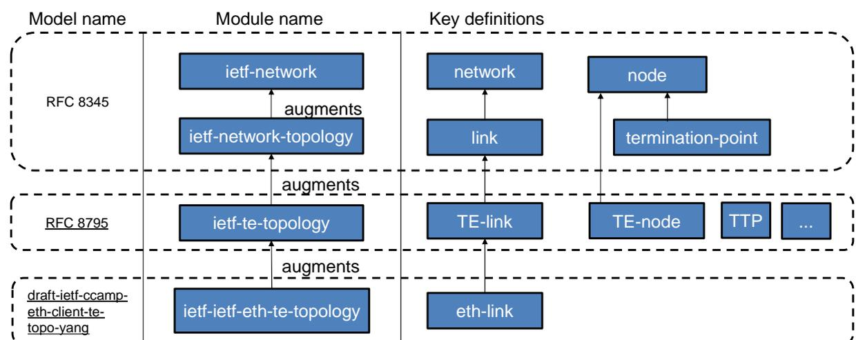
Figure 5.2.2.4.2: Ethernet Topology Model Hierarchy
