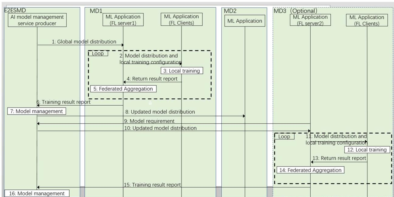
NOTE 1: Step 1 and step 6 are optional. Accordingly, initial global model used in FL process may be created by E2ESMD based on knowledge from other MDs or not.
