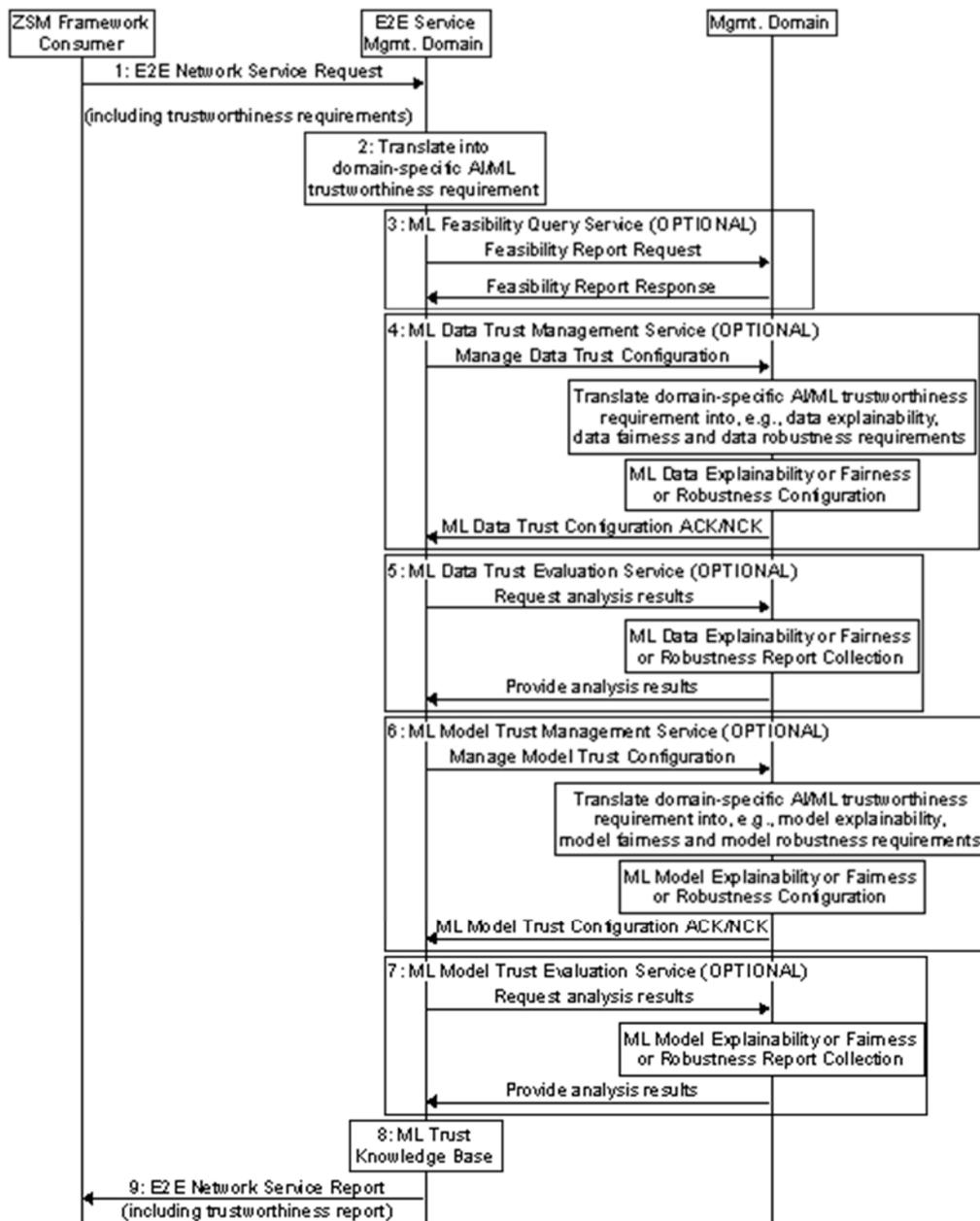
Figure A.1.3-1: Trustworthy ML workflow in ZSM framework
