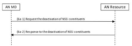
Figure 6.2.2.2.5-2: Example of a sequence of network slice subnet deactivation in AN MD
