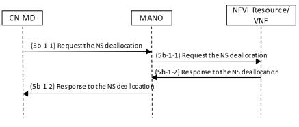
Figure 6.2.2.3-3: Example of a sequence of network slice subnet deallocation for resource in CN MD
