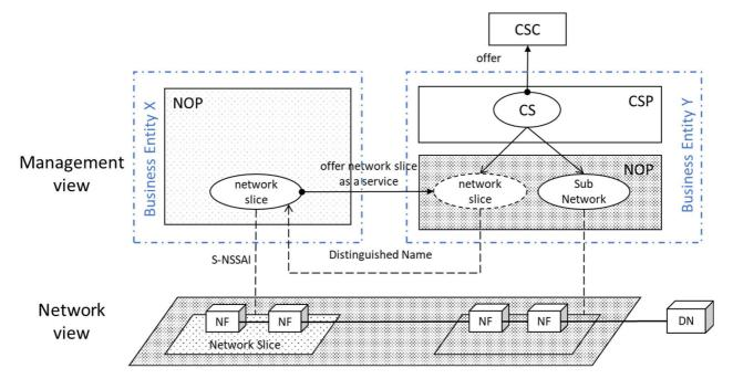
NOTE 1: Network slice shown on the left side of Figure 4.3.3-2 is a managed object instance created by NOP of Business Entity X. It is offered as a network slice as a service to Business Entity Y as a network slice shown on the right side of the same figure. CSP of Business Entity Y uses Distinguished Name to refer to and access the network slice created in the NOP.
