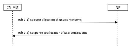
An example of a domain-level allocation sequence for OAM application in CN MD.
