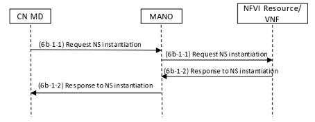
Figure 6.2.2.2.1-3: Example of a sequence of E2E network slice subnet allocation for resource in CN MD
