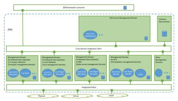
Figure B.1-1: Example of MDs to support network slicing using NFV
