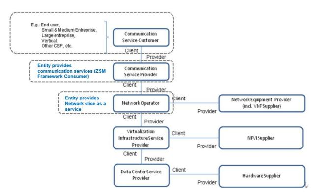
Figure 6.3.1-1: High-level model of roles for NSaaS
