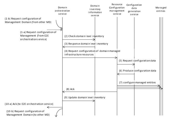
Figure C.1.2-1: Example of a domain-level sequence
