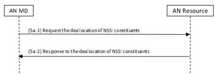
Figure 6.2.2.3-2: Example of a sequence of network slice subnet deallocation in AN MD
