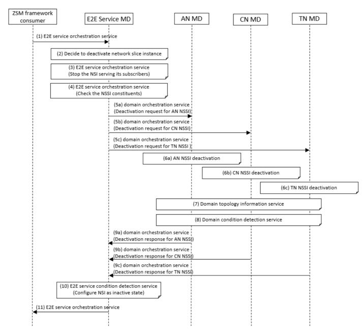
Figure 6.2.2.2.5-1: Deactivating network with E2E network slice for communication services
