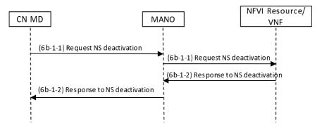
Figure 6.2.2.5-3: Example of a sequence of network slice subnet Deactivation for resource in CN MD
