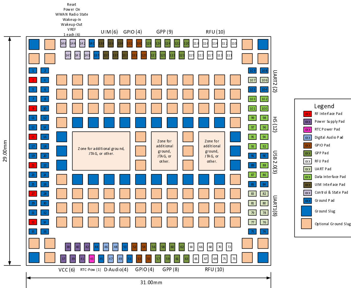
Figure 5: SMT3129 physical form factor (899 mm 2 ), dimensions, pad numbering and placement
