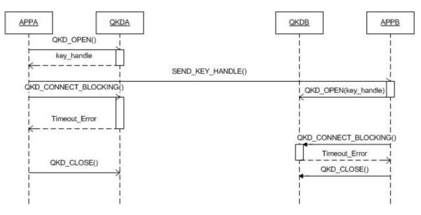
Figure 3: Case 2 - Undefined key handle and failed blocking call
