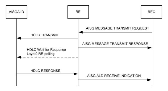
Figure 8.9.2-1: AISG Layer 7 message transfer in uplink and downlink - successful case
