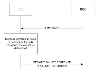
Figure 7.5-1: Default failure response upon malformed message
