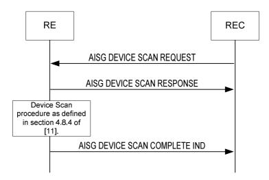
Figure 8.9.1-1: AISG Device Scan procedure
