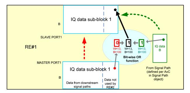
Figure 10.2.7.1-1: Bit wise OR function on input data for IQ data sub-block
