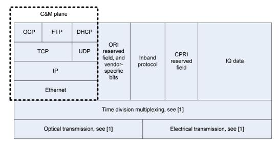
Figure 5.1-1: ORI protocol stack highlighting C&M plane
