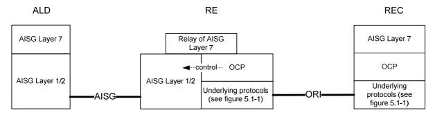
Figure 5.2.7-1: Protocol stack for OCP as a transport for AISG/3GPP luant Layer 7
