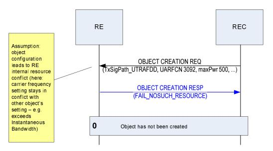
Figure 10.2.5.1-2: Sequence signal path setup failure
