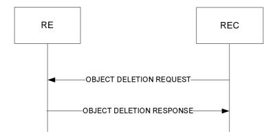
Figure 8.4.2-1: Object deletion procedure
