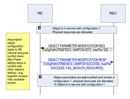
Figure 10.2.5.3-2: Sequence failed signal path modification
