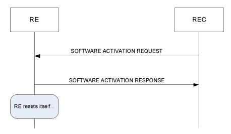
Figure 8.2.4.1-1: Software Activation procedure
