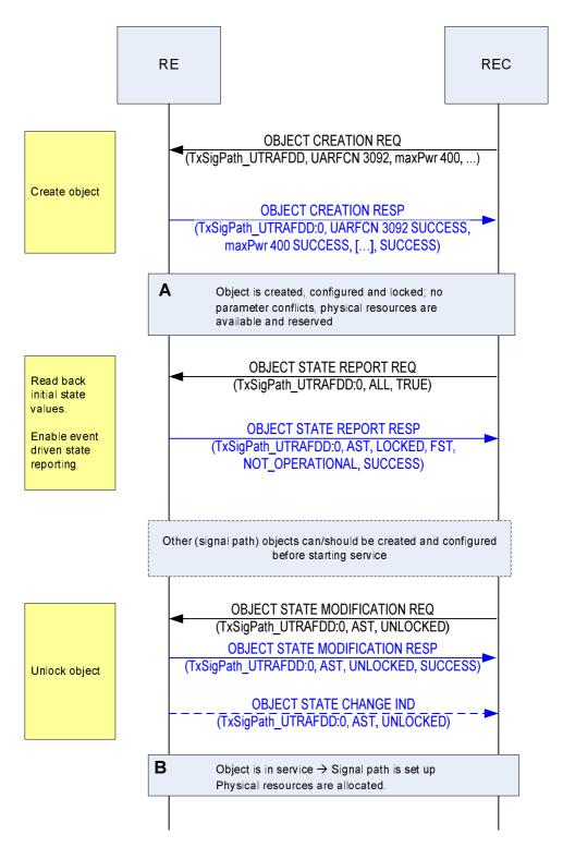
Figure 10.2.5.1-1: Sequence successful signal path setup
