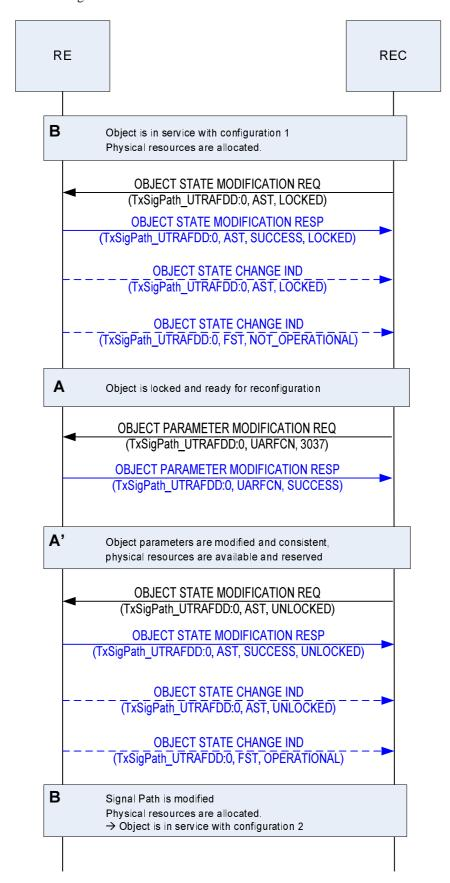
Figure 10.2.5.2-1: Sequence successful signal path modification
