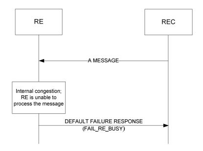
Figure 7.5-3: Default failure response upon internal congestion
