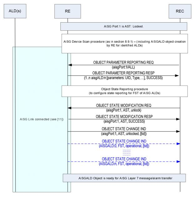
Figure 10.2.6.1.1-1: Layer 2 connection establishment using Device Scan procedure
