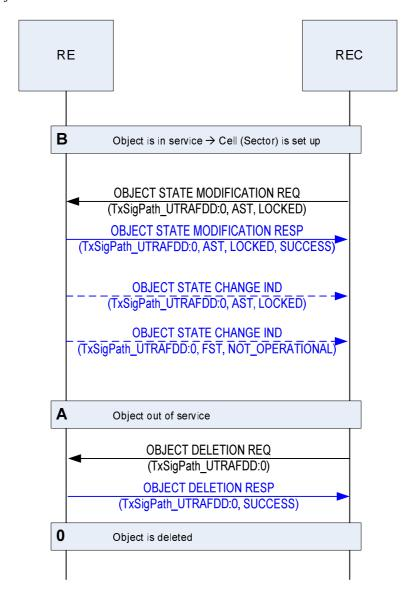
Figure 10.2.5.4-1: Sequence signal path deletion
