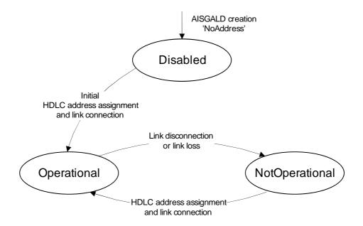
Figure 9.1.8-1: AISGALD FST state diagram
