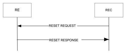
Figure 8.1.3-1: RE Reset procedure
