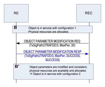
Figure 10.2.5.3-1: Sequence successful signal path modification
