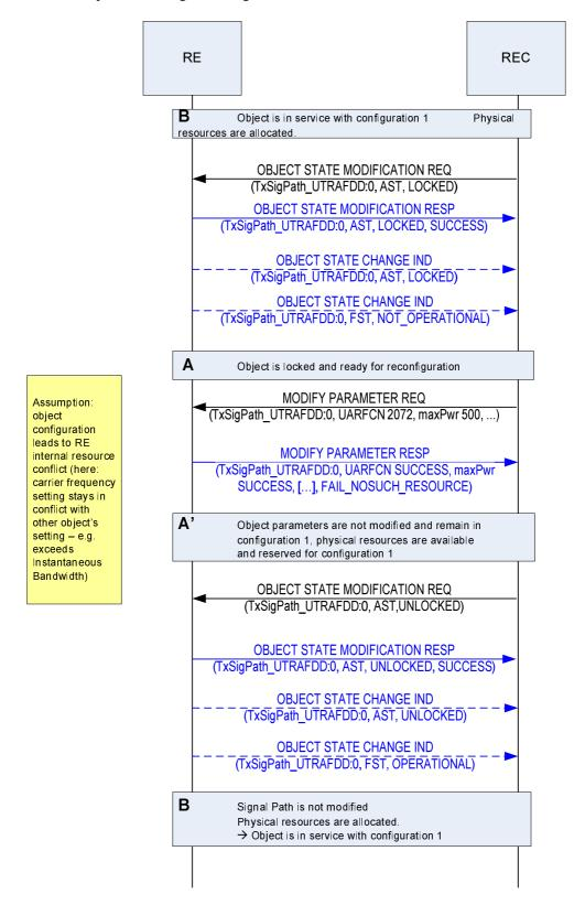
Figure 10.2.5.2-2: Sequence failed signal path modification
