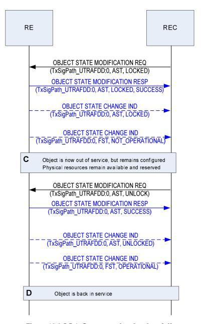
Figure 10.2.5.5-1: Sequence signal path on/off
