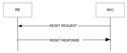
Figure 8.1.3-1: RE Reset procedure
