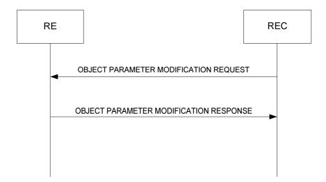
Figure 8.3.2-1: Object Parameter Modification procedure
