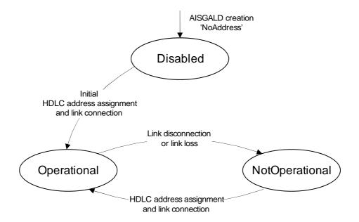
Figure 9.1.8-1: AISGALD FST state diagram
