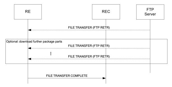
Figure 8.2.3-1: Software Download procedure
