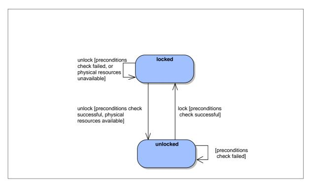
Figure 6.7.1.1-1: AST state transition diagram
