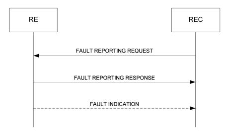
Figure 8.6.1-1: Fault Reporting procedure
