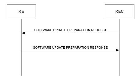
Figure 8.2.2-1: Software Update Preparation procedure
