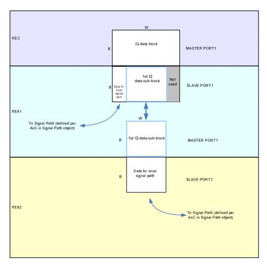
Figure 10.2.7.1-3: Chain configuration: different line bit rates on ORI links terminating at the master and slave ports
