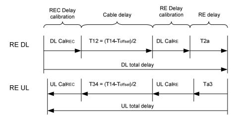
Figure 10.2.4-2: Relation of time components for single-hop and multi-hop
