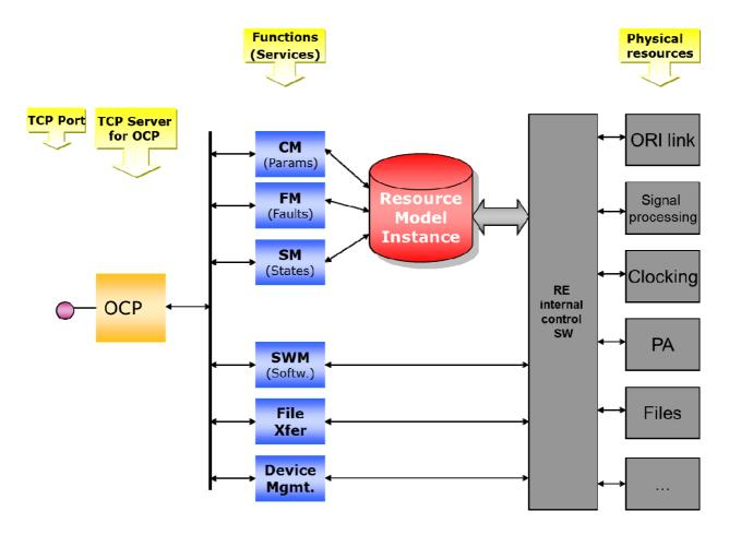
Figure 6.1-1: System view of the Resource Model
