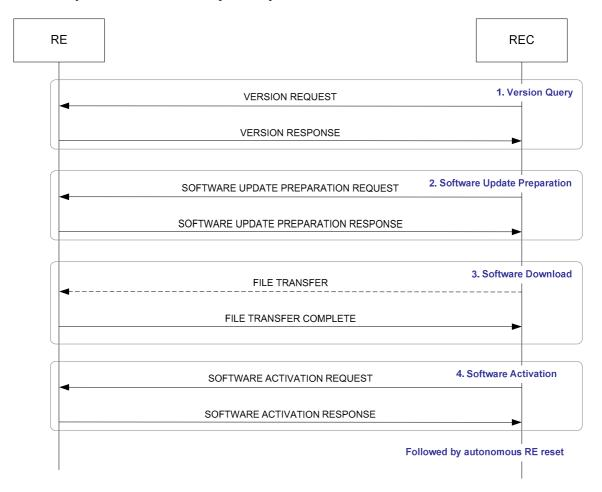
Figure 10.1.3.3-1: RE Software Alignment
