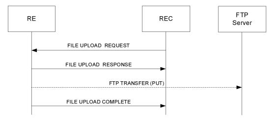
Figure 8.8.2-1: File Upload procedure
