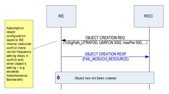
Figure 10.2.5.1-2: Sequence signal path setup failure
