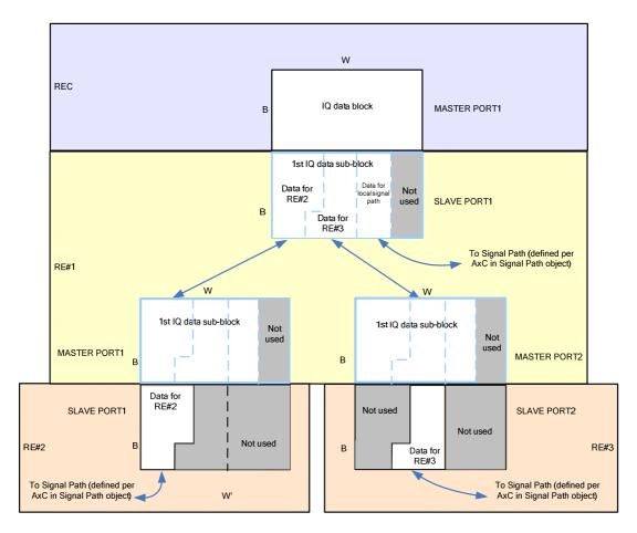
Figure 10.2.7.1-4: Tree configuration: identical line bit rates on ORI links terminating at the master and slave ports
