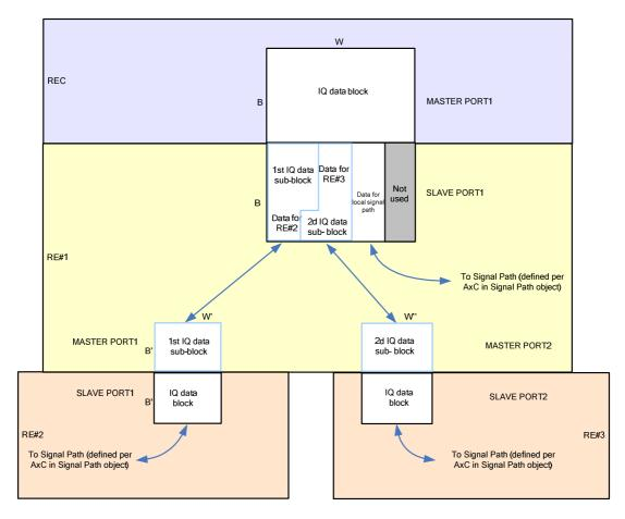
Figure 10.2.7.1-5: Tree configuration: different line bit rates on ORI links terminating at the master and slave ports
