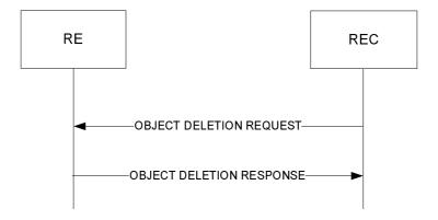
Figure 8.4.2-1: Object deletion procedure
