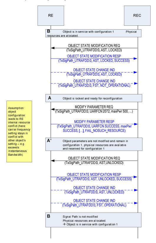
Figure 10.2.5.2-2: Sequence failed signal path modification
