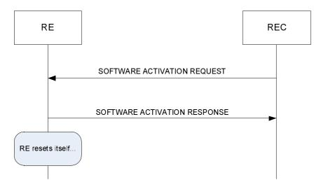
Figure 8.2.4.1-1: Software Activation procedure
