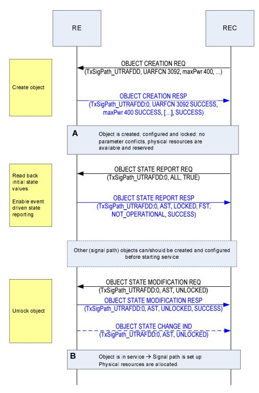
Figure 10.2.5.1-1: Sequence successful signal path setup
