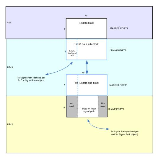
Figure 10.2.7.1-2: Chain configuration: identical line bit rates on ORI links terminating at the master and slave ports
