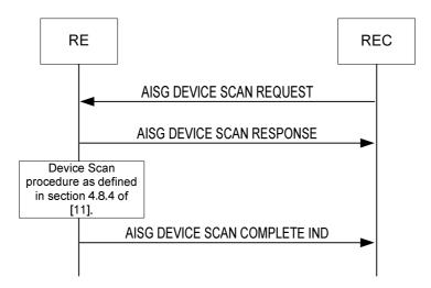
Figure 8.9.1-1: AISG Device Scan procedure
