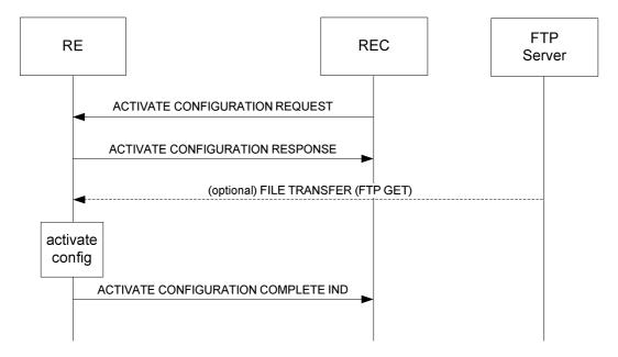
Figure 8.8.3-1: Activate Configuration procedure
