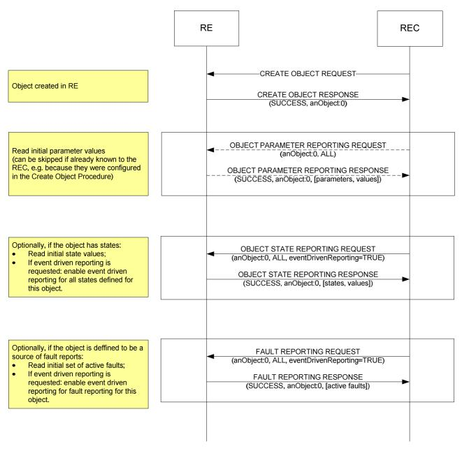
Figure 10.2.1-1: Dynamic object initial status alignment
