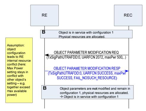
Figure 10.2.5.3-2: Sequence failed signal path modification
