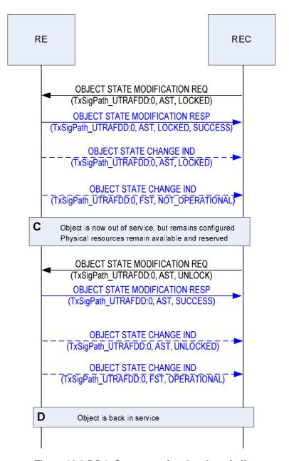
Figure 10.2.5.5-1: Sequence signal path on / off
