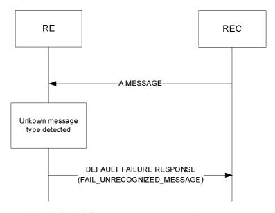
Figure 7.5-2: Default failure response upon unknown message type
