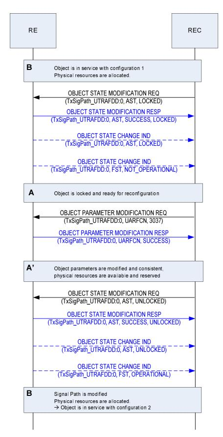
Figure 10.2.5.2-1: Sequence successful signal path modification
