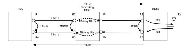
Figure 10.2.4-1a: Time components for multi-hop
