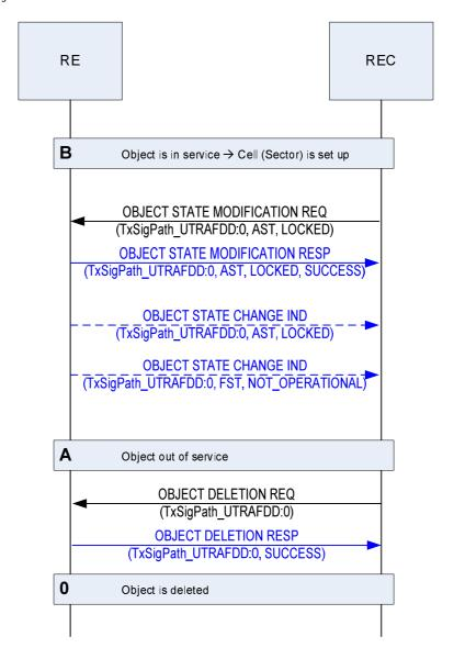
Figure 10.2.5.4-1: Sequence signal path deletion
