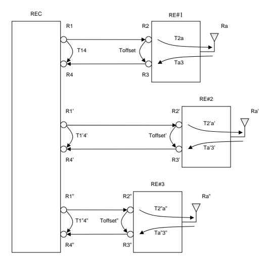
Figure 10.2.4-1: Time components for single hop
