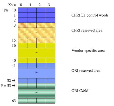
Figure 6.1.1: Control word mapping to subchannel allocation
