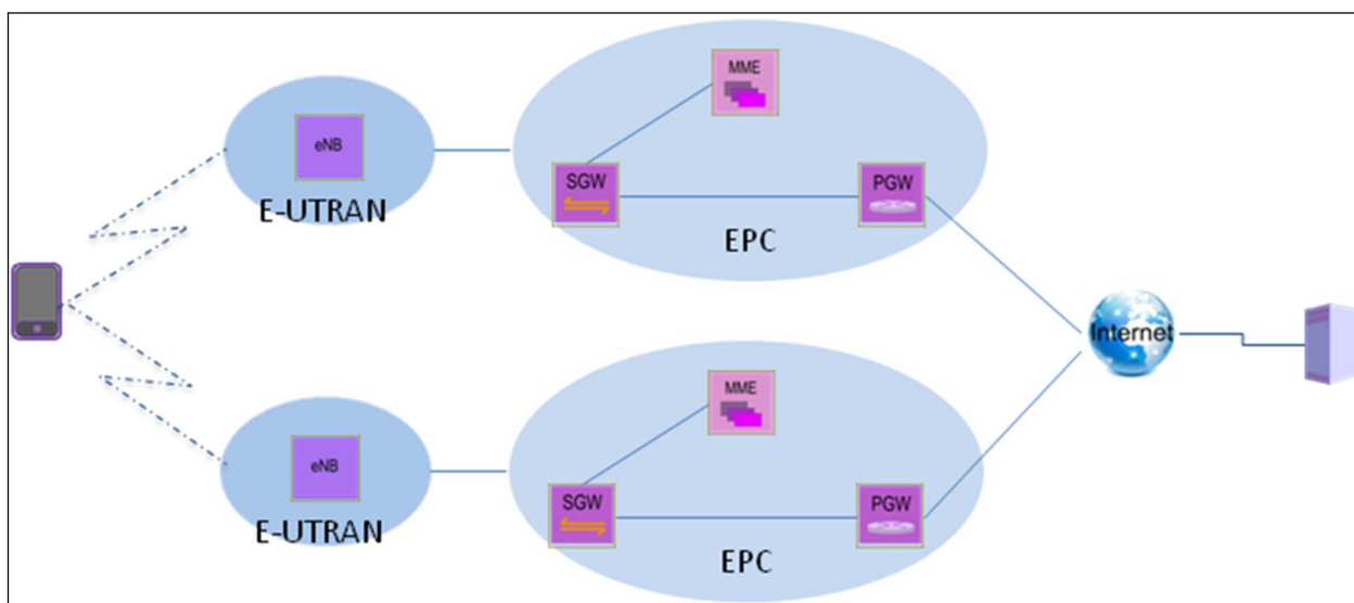
Figure 20: UE communicates with a fixed device; UE is moving across different P-GW domain
