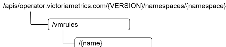
Figure 10.3-1: Resource URI structure of VMRule resource object for the Metrics Analysis Exposure interface
