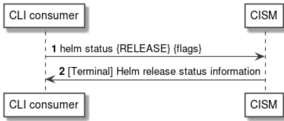
Figure 7.3.5-1: Flow of containerized workload information querying
