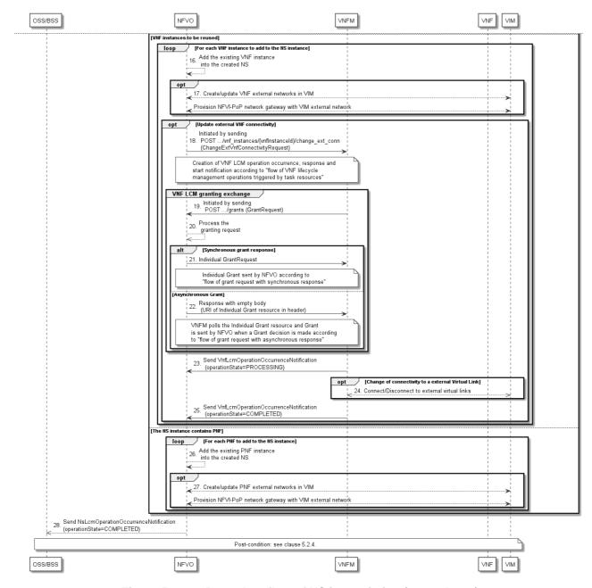
Figure 5.2.3-2: Procedure flow of NS instantiation (second part)
