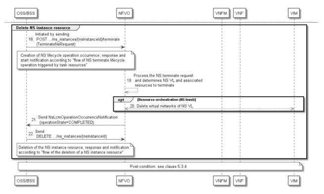
Figure 5.3.3.2-2: Procedure of NS termination by terminating individual NS constituents (second part)
