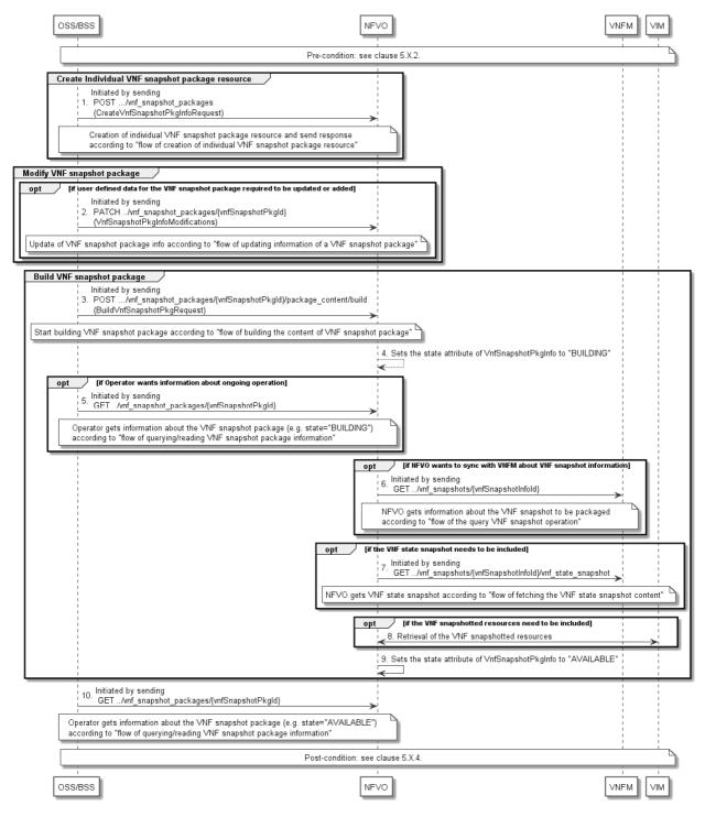
Figure 5.7.3-1: Procedure flow of VNF snapshot package creation
