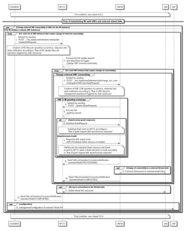
Figure 5.5.3-1: Procedure flow of NS update changing the external VNF connectivity
