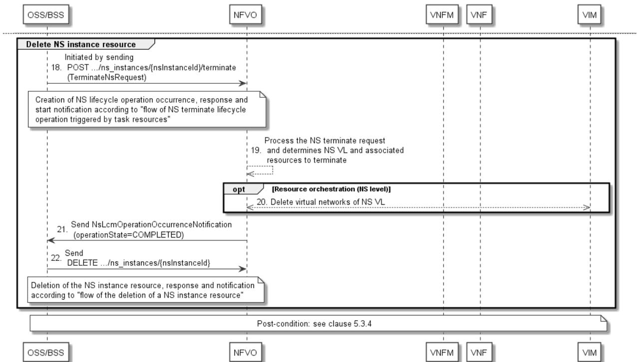
**Figure 5.3.3.2-2: Procedure of NS termination by terminating individual NS constituents (second part)**
