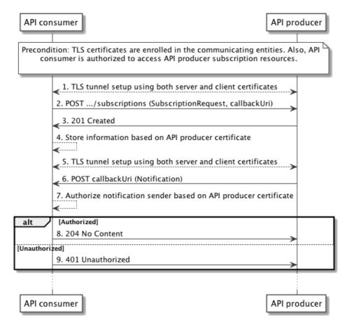
Figure 8.2.6-1: Authorization of notifications using TLS certificates
