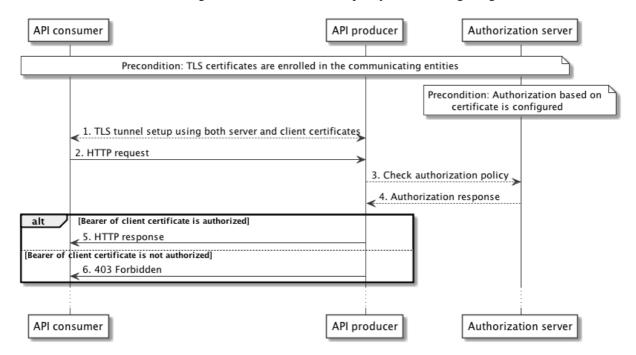
Figure 8.2.3-1: Authorization of API requests using TLS certificates
