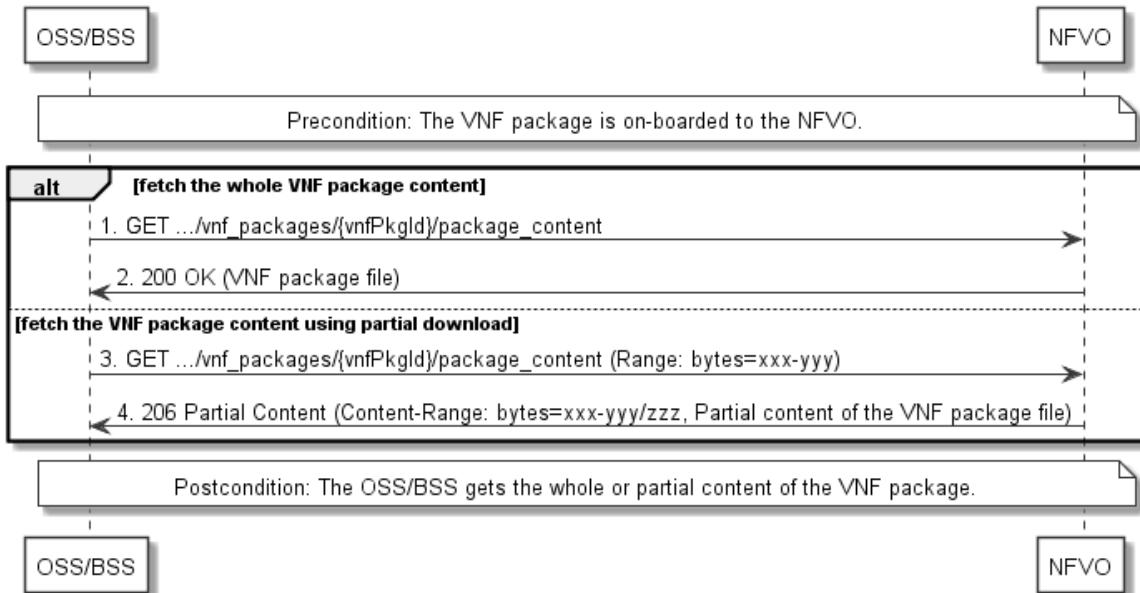
**Figure 9.3.7-1: Flow of fetching an on-boarded VNF package**
