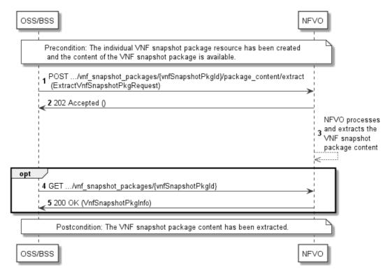
Figure 11.3.9-1: Flow of extracting the content of a VNF snapshot package
