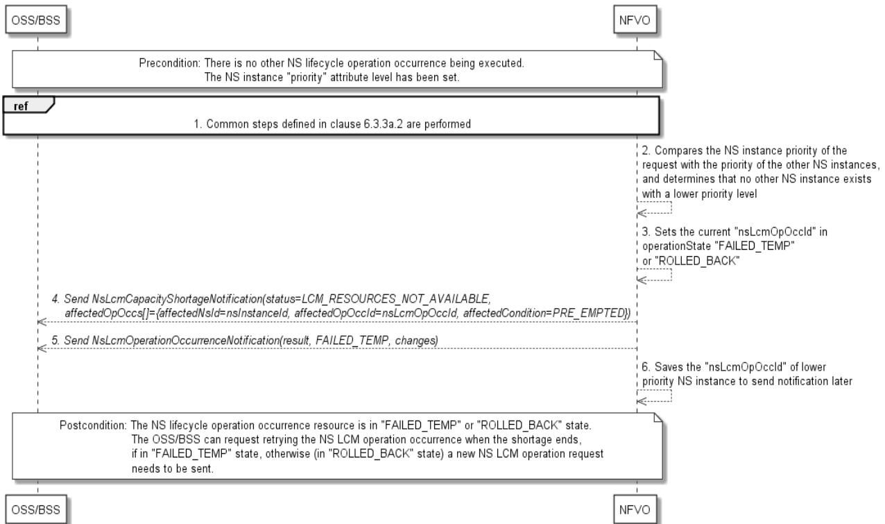
**Figure 6.3.3a.3-1: Flow of Shortage use case #1**
