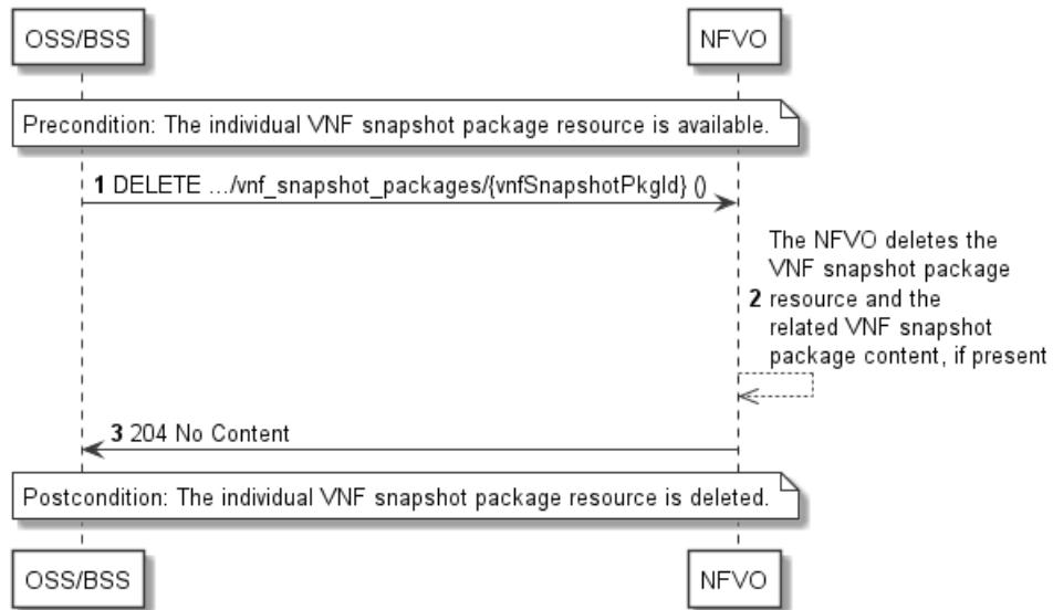
**Figure 11.3.4-1: Flow of deleting a VNF package resource**
