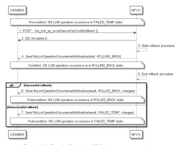
Figure 6.3.8-1: Flow of rolling back an NS lifecycle management operation
