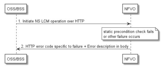
Figure 6.6.3.1-1: Immediate failure of an NS LCM operation
