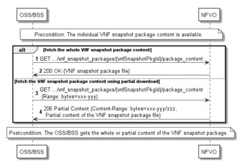
Figure 11.3.6-1: Flow of fetching a VNF snapshot package
