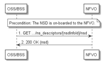
Figure 5.3.6a-1: Flow of reading an NSD
