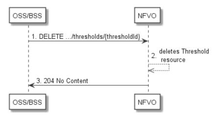
Figure 7.3.7-1: Flow of threshold deletion
