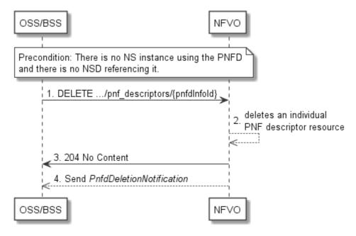
Figure 5.3.10-1: Flow of the deletion of an individual PNF descriptor resource
