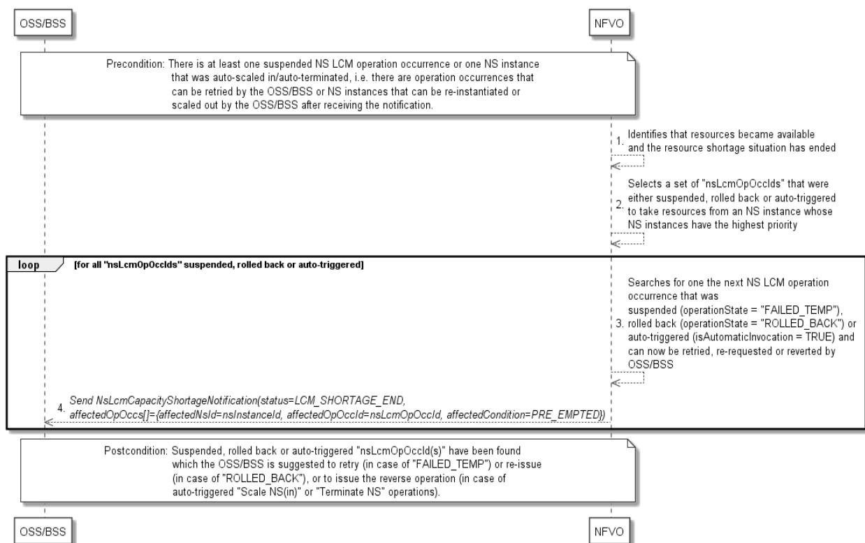
Figure 6.3.3a.6-1: Flow of Shortage use case #4
