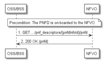
Figure 5.3.11a-1: Flow of reading a PNFD
