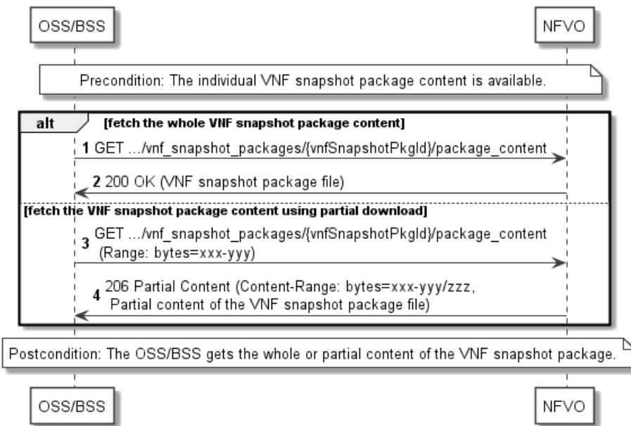
**Figure 11.3.6-1: Flow of fetching a VNF snapshot package**
