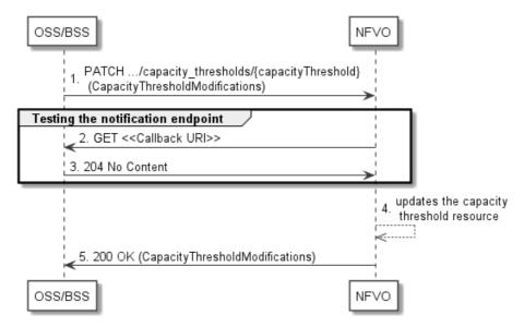
Figure 10.3.5-1: Flow of updating the callback URI of a threshold
