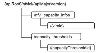
Figure 10.2-1: Resource URI structure of the NFVI Capacity Information interface
