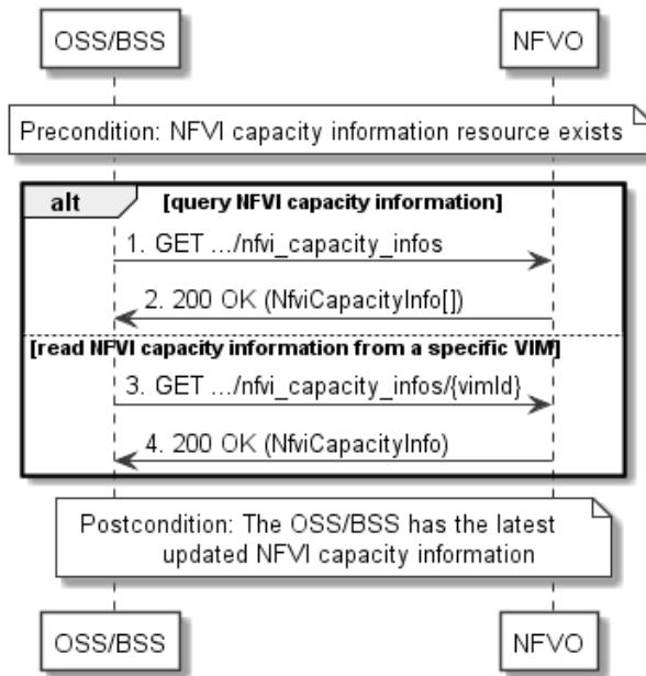
**Figure 10.3.1-1: Flow of querying/reading NFVI capacity information**
