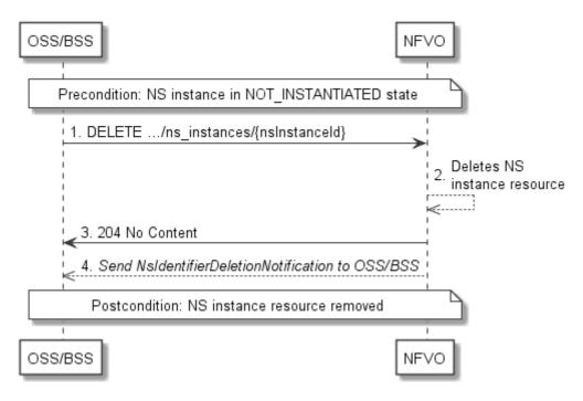
Figure 6.3.2-1: Flow of the deletion of an NS instance resource
