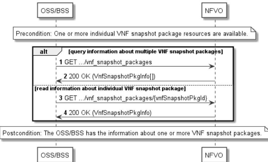
**Figure 11.3.2-1: Flow of querying/reading VNF snapshot package information**
