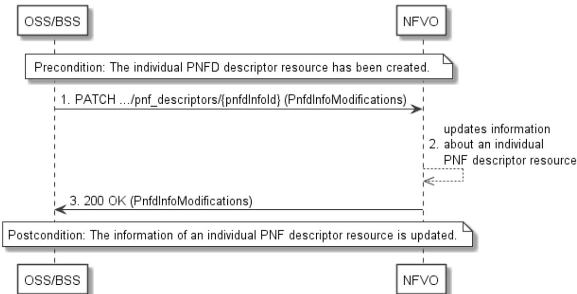
**Figure 5.3.9a-1: Flow of the update of an individual PNF descriptor resource**
