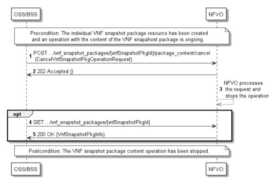
Figure 11.3.10-1: Flow of cancelling the operation with the VNF snapshot package content
