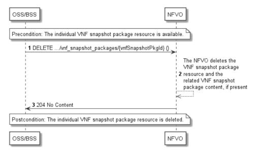
Figure 11.3.4-1: Flow of deleting a VNF package resource
