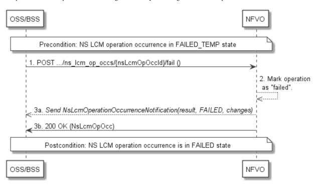
Figure 6.3.10-1: Flow of declaring an NS lifecycle management operation as failed
