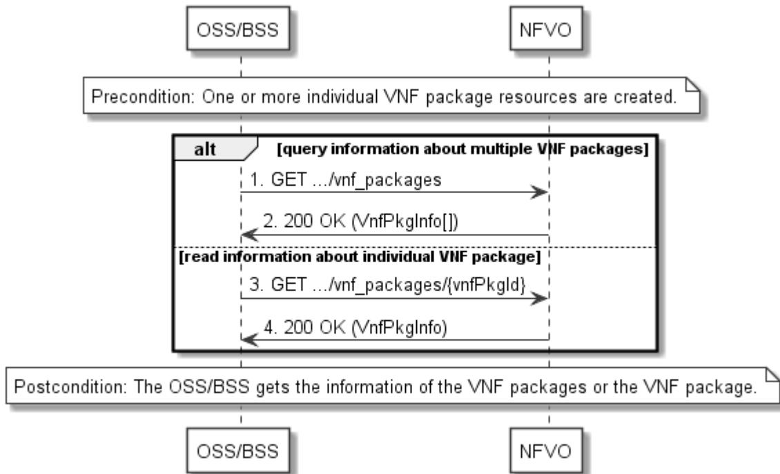
**Figure 9.3.3-1: Flow of querying/reading VNF package information**
