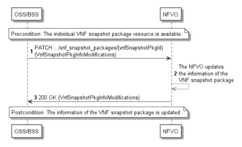
Figure 11.3.3-1: Flow of updating information of a VNF snapshot package
