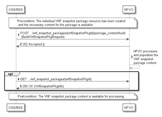
Figure 11.3.8-1: Flow of building the content of VNF snapshot package
