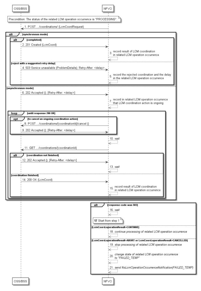
Figure 12.3.1-1: Flow of LCM coordination
