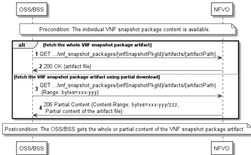
**Figure 11.3.7-1: Flow of fetching a VNF snapshot package artifact**
