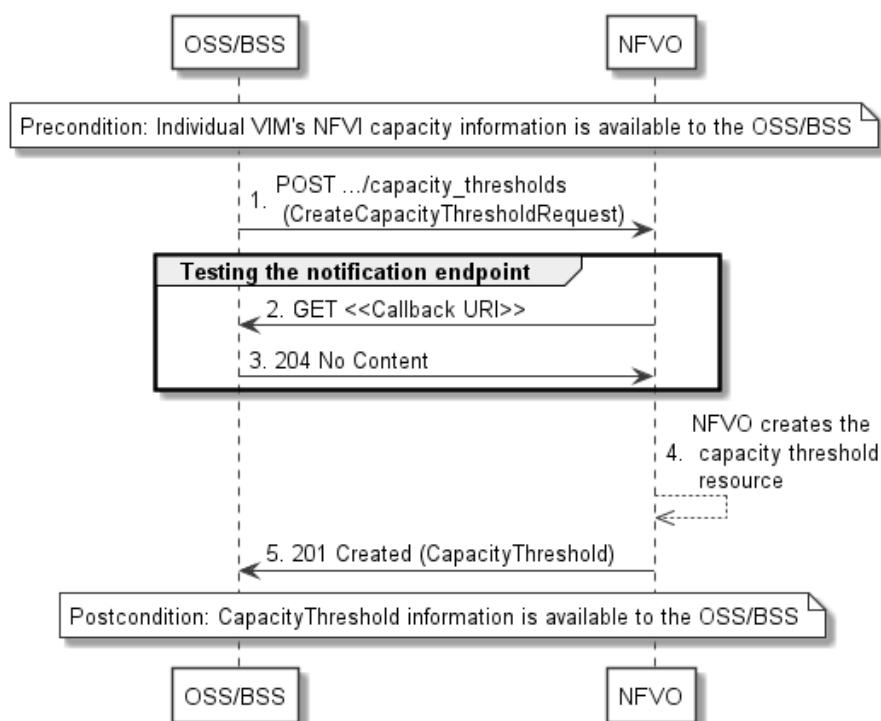
**Figure 10.3.2-1: Flow of creating a capacity threshold**
