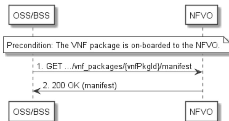
**Figure 9.3.2b-1: Flow of fetching the VNF package manifest**
