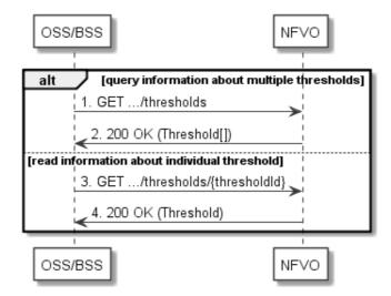
Figure 7.3.6-1: Flow of thresholds query/read
