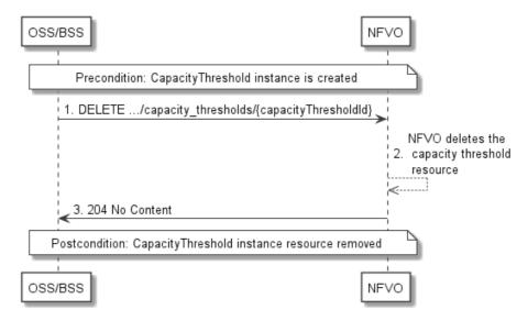
Figure 10.3.4-1: Flow of capacity threshold deletion
