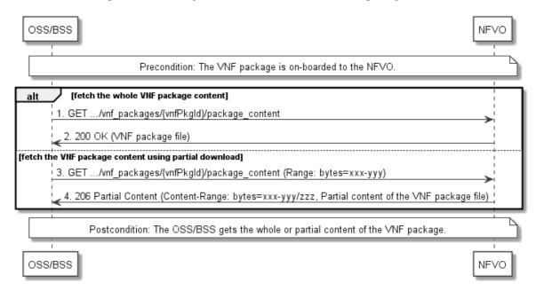
Figure 9.3.7-1: Flow of fetching an on-boarded VNF package
