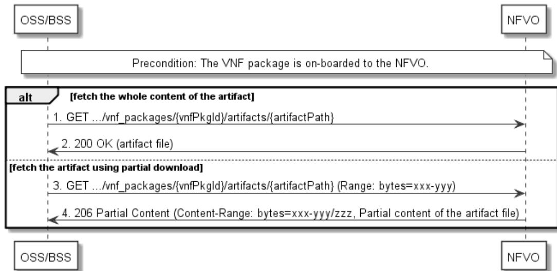
**Figure 9.3.8-1: Flow of fetching a VNF package artifact**
