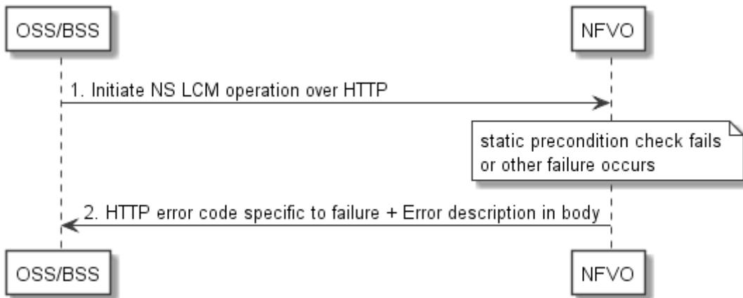
**Figure 6.6.3.1-1: Immediate failure of an NS LCM operation**
