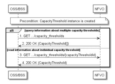
Figure 10.3.3-1: Flow of capacity thresholds query/read
