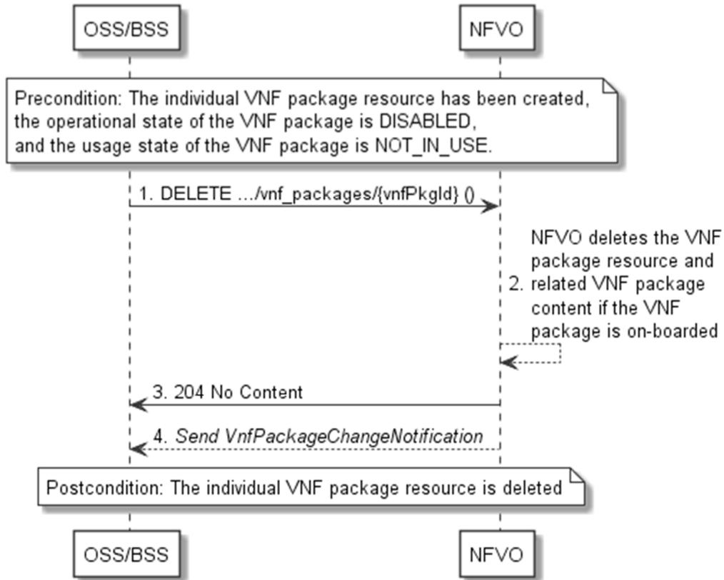
**Figure 9.3.6-1: Flow of deleting a VNF package resource**
