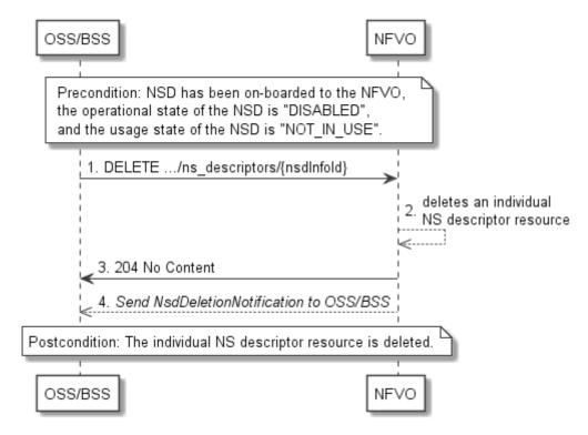
Figure 5.3.5-1: Flow of the deletion of an individual NS descriptor resource
