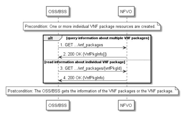
Figure 9.3.3-1: Flow of querying/reading VNF package information
