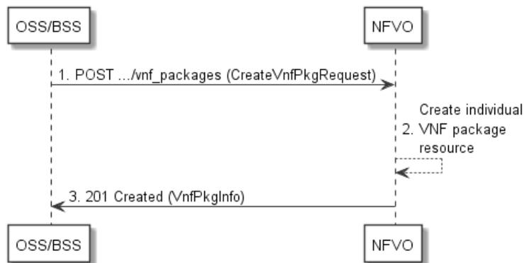
**Figure 9.3.1-1: Flow of the creation of an individual VNF package resource**
