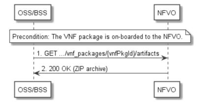
Figure 9.3.4a-1: Flow of bulk-fetching VNF package artifacts
