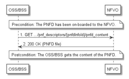
Figure 5.3.9-1: Flow of the fetching of PNFD content
