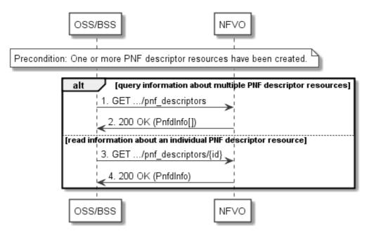
Figure 5.3.11-1: Flow of the querying/reading of PNF descriptor resources
