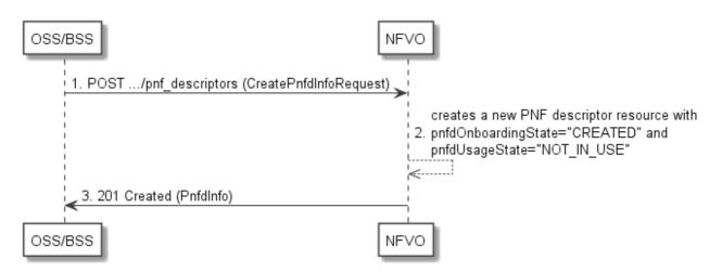
Figure 5.3.7-1: Flow of the creation of an individual PNF descriptor resource
