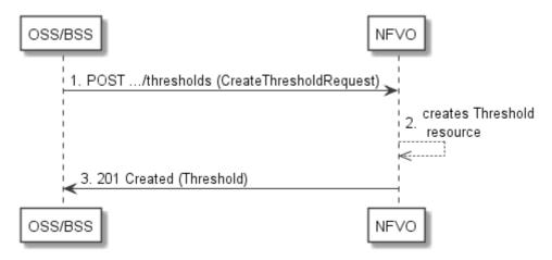
Figure 7.3.5-1: Flow of threshold creation
