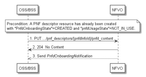
Figure 5.3.8-1: Flow of the uploading of PNFD content
