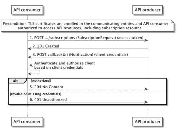
Figure 4.5.2.2-1: Authorization of notifications using the HTTP Basic authentication scheme
