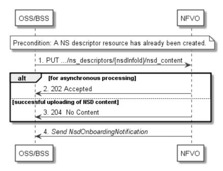
Figure 5.3.2-1: Flow of the uploading of NSD content
