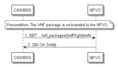
Figure 9.3.4-1: Flow of reading VNFD
