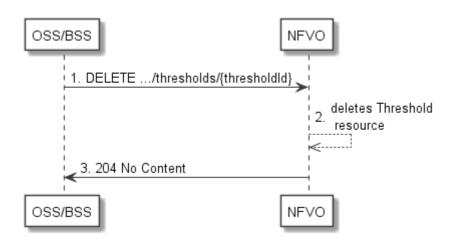
Figure 7.3.7-1: Flow of threshold deletion
