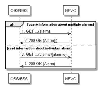
Figure 8.3.1-1: Flow of alarm query/read
