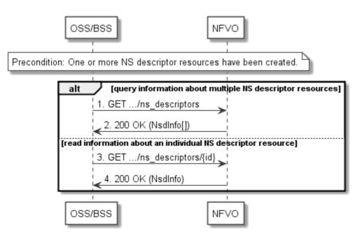
Figure 5.3.6-1: Flow of the querying/reading of NS descriptor resources
