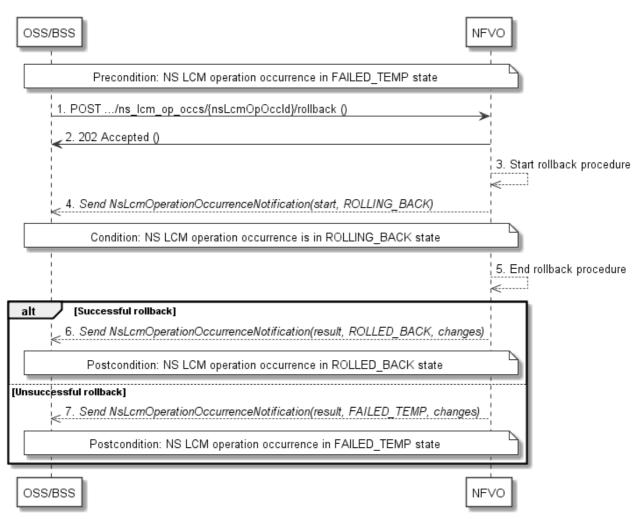
Figure 6.3.8-1: Flow of rolling back a NS lifecycle management operation
