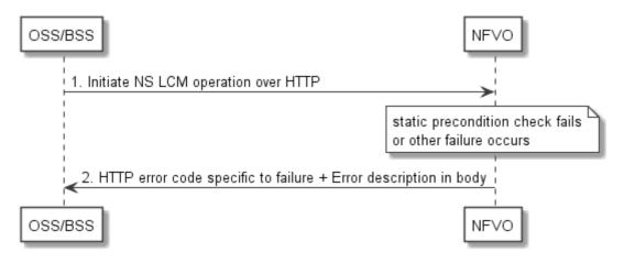
Figure 6.6.3.1-1: Immediate failure of a NS LCM operation
