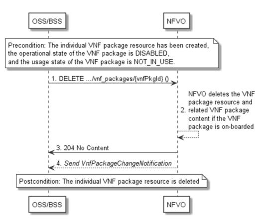
Figure 9.3.6-1: Flow of deleting a VNF package resource
