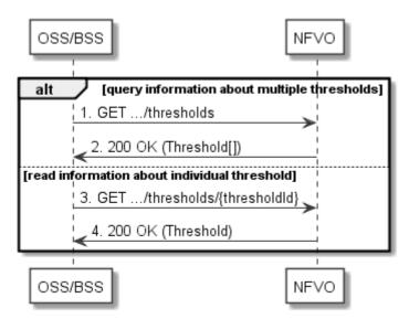
Figure 7.3.6-1: Flow of thresholds query/read
