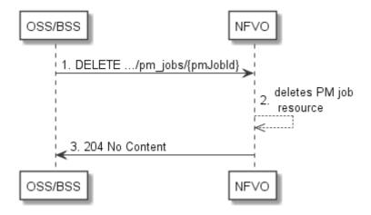
Figure 7.3.3-1: Flow of PM job deletion
