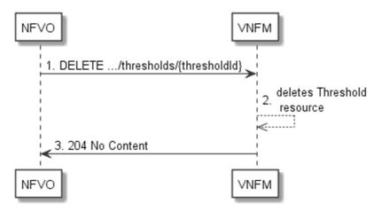
Figure 6.3.7-1: Flow of threshold deletion
