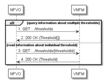
Figure 6.3.6-1: Flow of thresholds query/read
