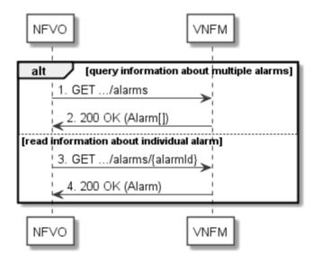
Figure 7.3.1-1: Flow of alarm query/read
