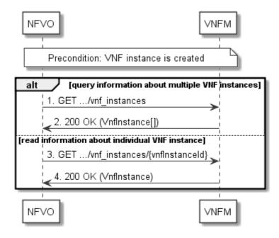
Figure 5.3.5-1: Flow of VNF instance query/read
