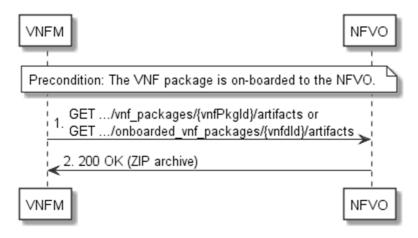
Figure 10.3.4a-1: Flow of bulk-fetching VNF package artifacts
