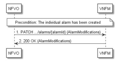
Figure 7.3.2-1: Flow of acknowledging alarm
