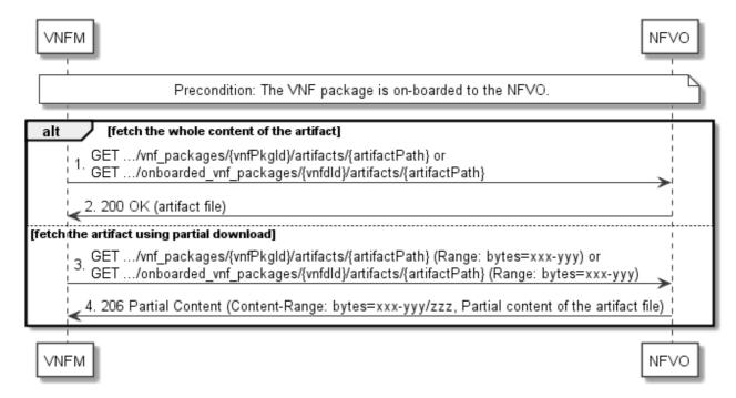
Figure 10.3.4-1: Flow of fetching a VNF package artifact
