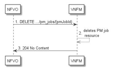
Figure 6.3.3-1: Flow of PM job deletion
