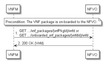
Figure 10.3.2-1: Flow of reading VNFD
