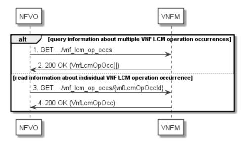
Figure 5.3.7-1: Flow of Get VNF lifecycle operation status
