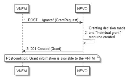
Figure 9.3.1-1: Flow of granting with synchronous response
