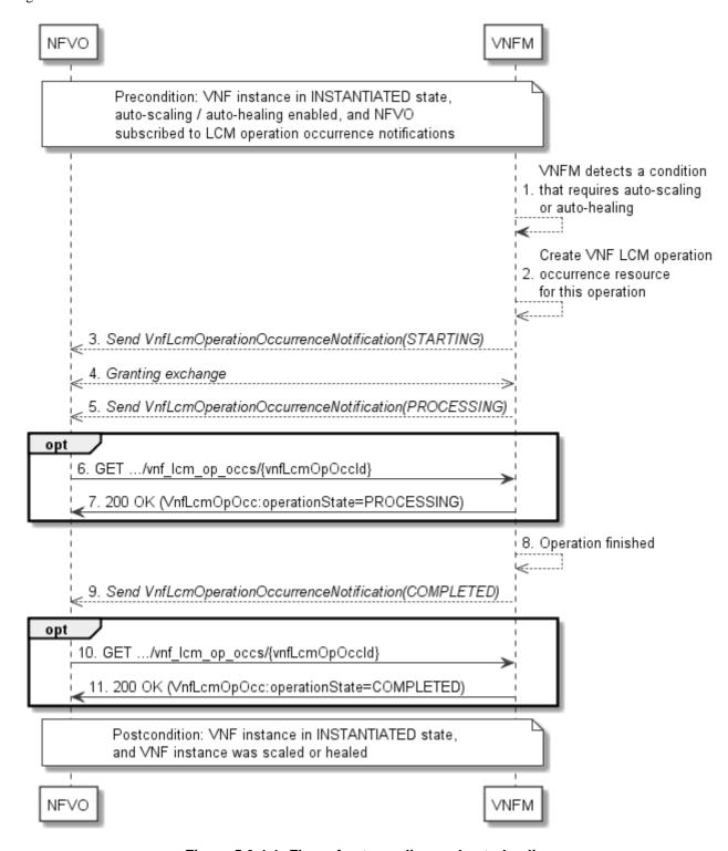
Figure 5.3.4-1: Flow of auto-scaling and auto-healing
