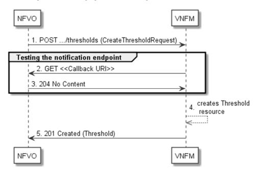
Figure 6.3.5-1: Flow of threshold creation
