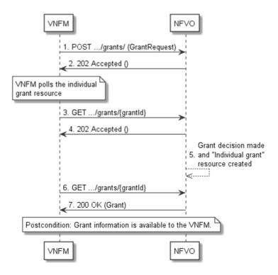
Figure 9.3.2-1: Flow of granting with asynchronous response
