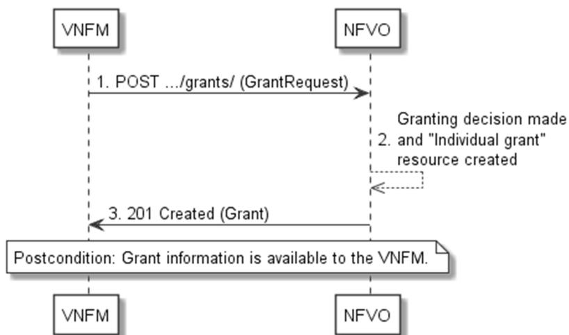
**Figure 9.3.1-1: Flow of granting with synchronous response**
