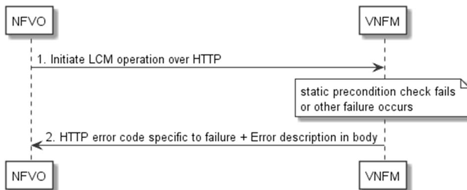
**Figure 5.6.3.1-1: Immediate failure of a VNF LCM operation**
