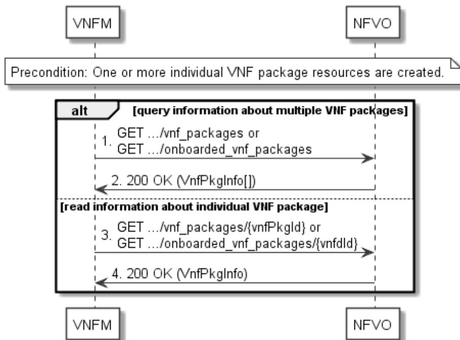
**Figure 10.3.1-1: Flow of querying/reading VNF package information**
