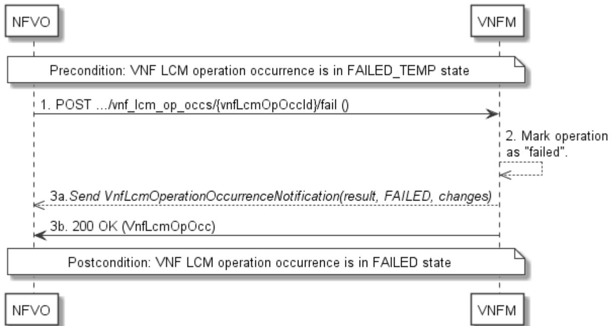
**Figure 5.3.12-1: Flow of declaring a VNF lifecycle management operation as failed**
