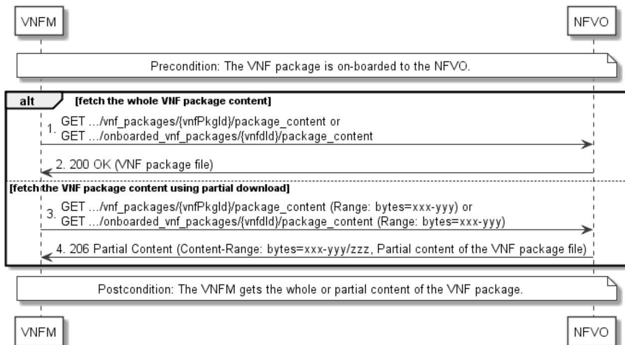
**Figure 10.3.3-1: Flow of fetching an on-boarded VNF package**
