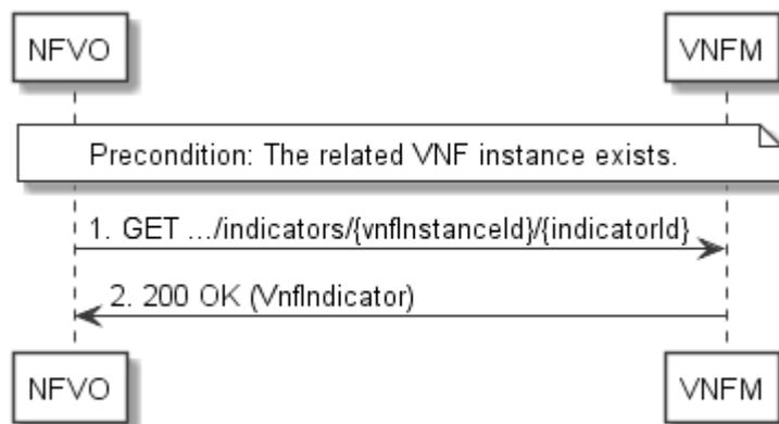
**Figure 8.3.2-1: Flow of reading a VNF indicator**
