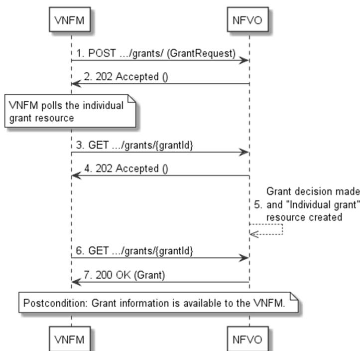
**Figure 9.3.2-1: Flow of granting with asynchronous response**
