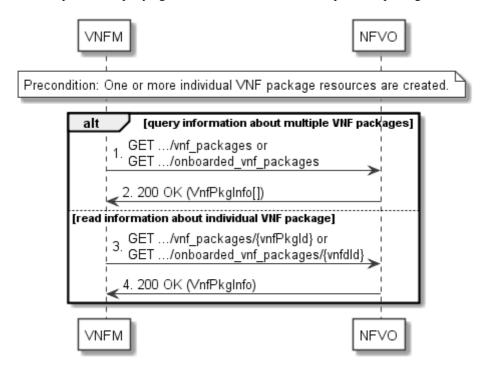
Figure 10.3.1-1: Flow of querying/reading VNF package information
