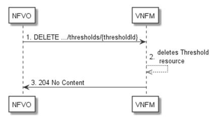
Figure 6.3.7-1: Flow of threshold deletion
