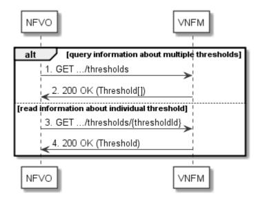
Figure 6.3.6-1: Flow of thresholds query/read
