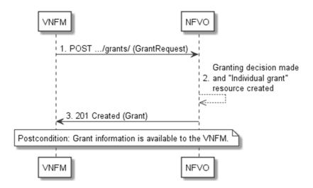
Figure 9.3.1-1: Flow of granting with synchronous response
