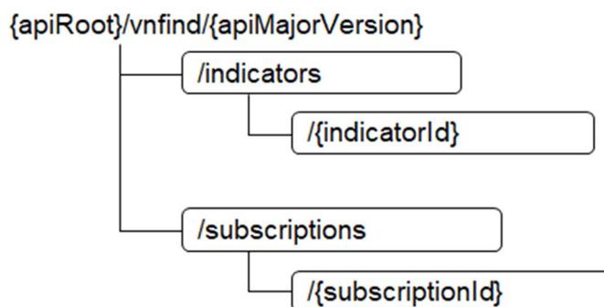
**Figure 8.2-2: Resource URI structure of the VNF Indicator Interface exposed by the VNF**
