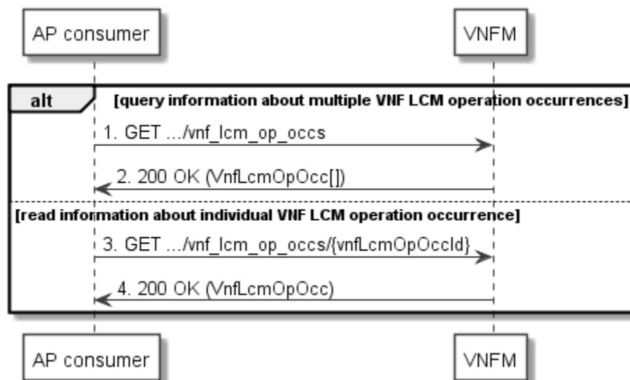
**Figure 5.3.7-1: Flow of Get VNF lifecycle operation status**
