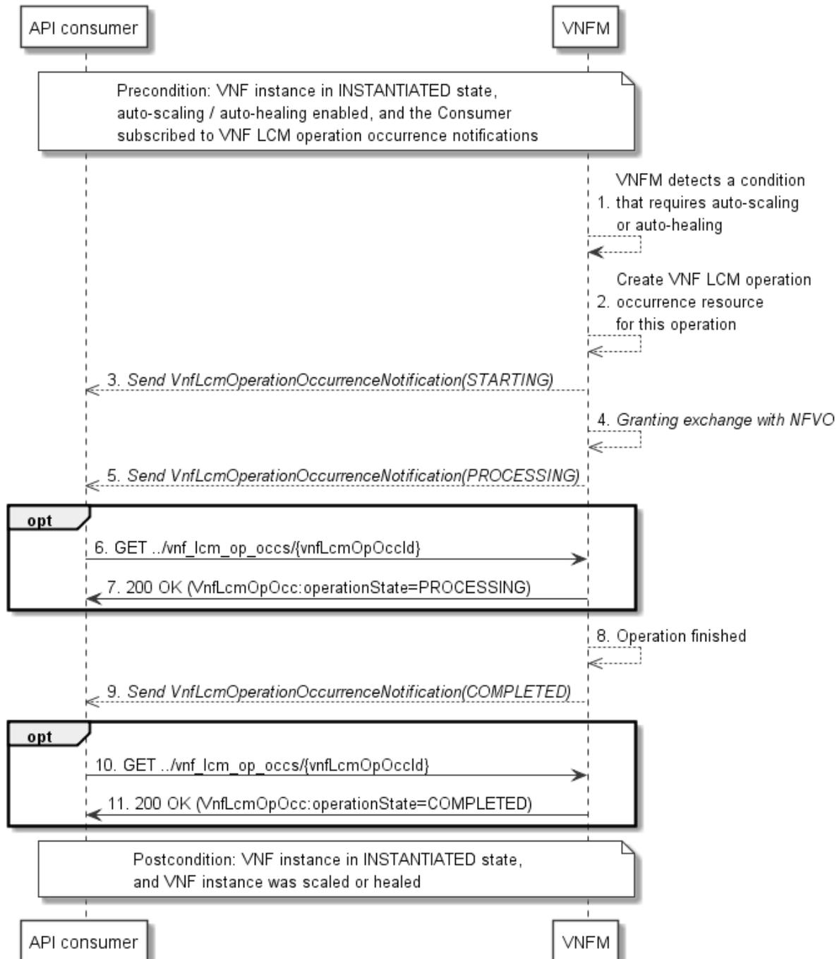
**Figure 5.3.4-1: Flow of auto-scaling and auto-healing**
