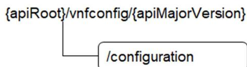
**Figure 9.2-1: Resource URI structure of VNF configuration Interface**
