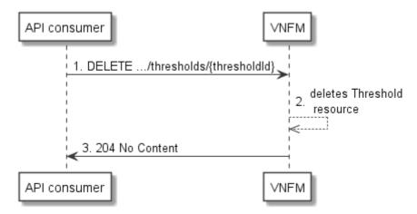
Figure 6.3.7-1: Flow of threshold deletion
