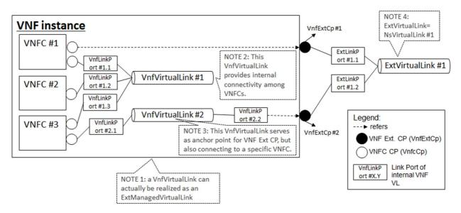
Figure B.3.2-1: Example of a VNF instance with two different types of external connection points
