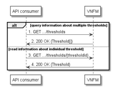
Figure 6.3.6-1: Flow of thresholds query/read
