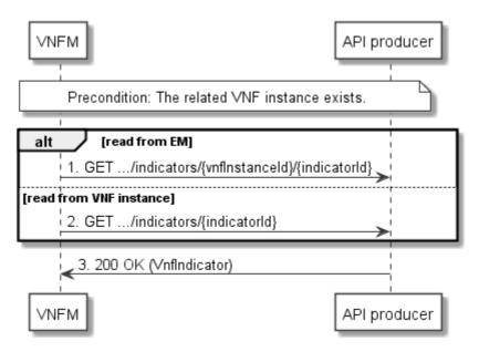
Figure 8.3.2-1: Flow of reading a VNF indicator
