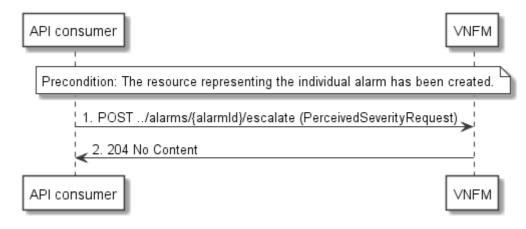
Figure 7.3.2-1: Escalate perceived severity task flow
