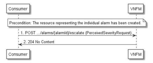
Figure 7.3.2-1: Escalate perceived severity task flow
