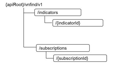
Figure 8.2-2: Resource URI structure of the VNF Indicator Interface exposed by the VNF
