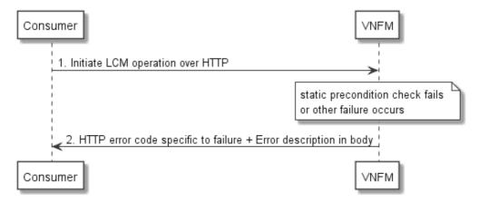
Figure 5.6.3.1-1: Immediate failure of a VNF LCM operation
