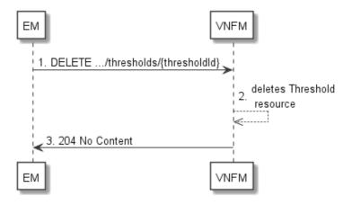
Figure 6.3.7-1: Flow of threshold deletion
