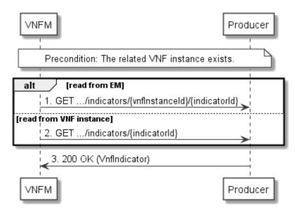
Figure 8.3.2-1: Flow of reading a VNF indicator
