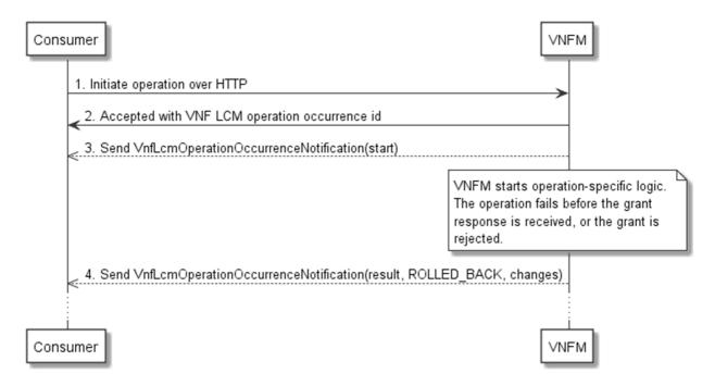
Figure 5.6.3.2-1: Failure of a VNF LCM operation before applying any change to the VNF instance
