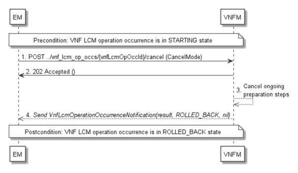
Figure 5.3.13-1: Flow of cancelling a VNF lifecycle management operation in "STARTING" state
