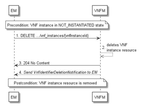
Figure 5.3.2-1: Flow of the deletion of a VNF instance resource
