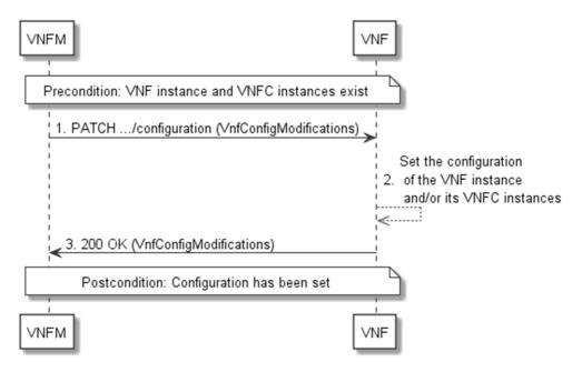
Figure 9.3.1-1: Flow of setting the configuration of a VNF instance and/or its VNFC instances
