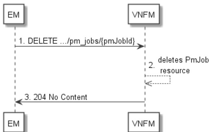
**Figure 6.3.3-1: Flow of PM job deletion**
