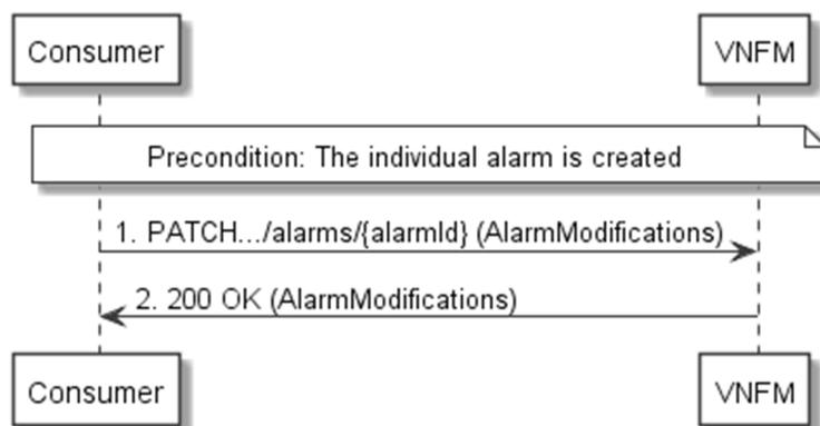
**Figure 7.3.3-1: Flow of acknowledging alarm**
