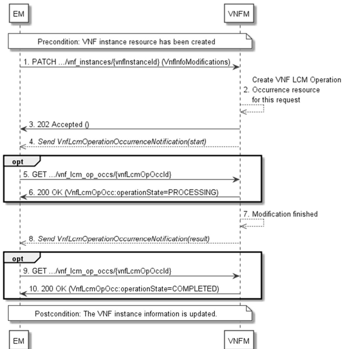
**Figure 5.3.6-1: Flow of the modification of VNF instance information**
