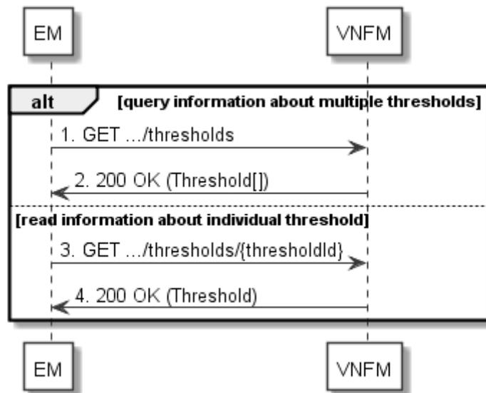
**Figure 6.3.6-1: Flow of thresholds query/read**
