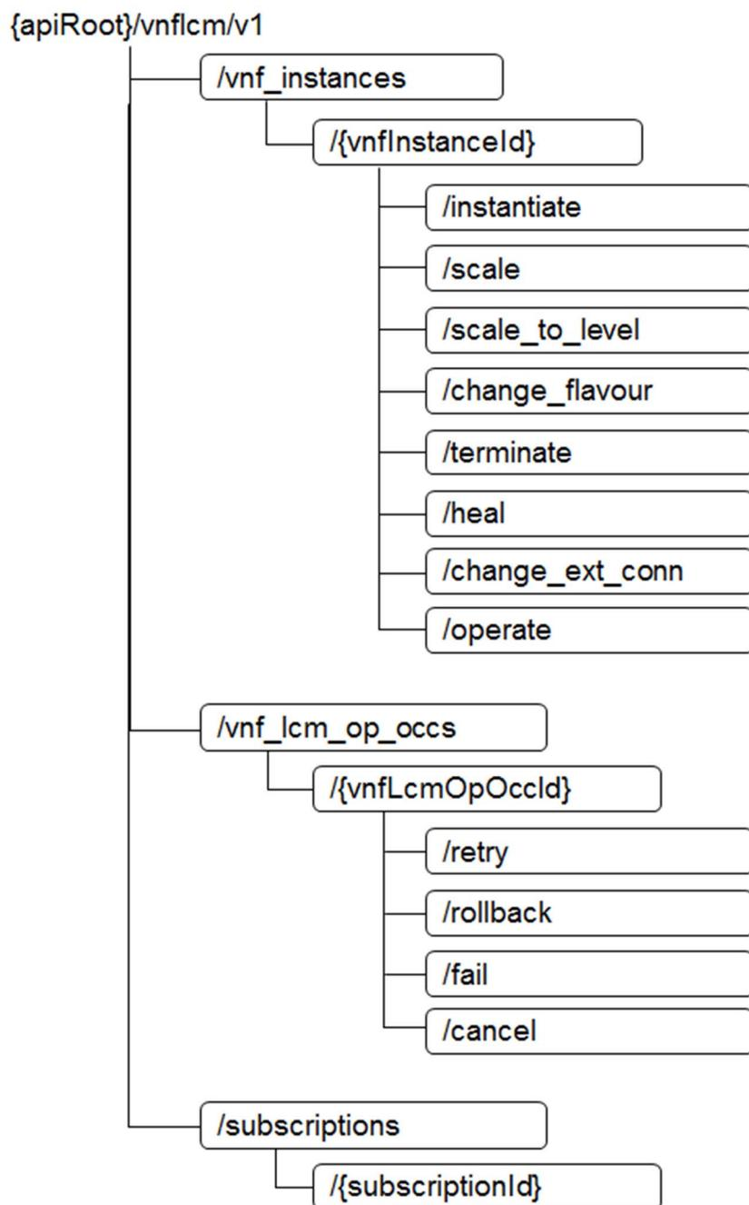
Figure 5.2-1: Resource URI structure of the VNF Lifecycle Management Interface
