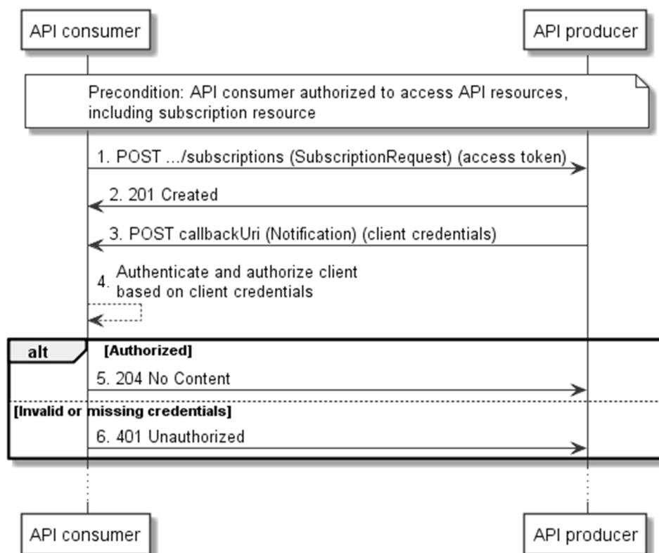
Figure 4.5.2.2-1: Authorization of notifications using the HTTP Basic authentication scheme
