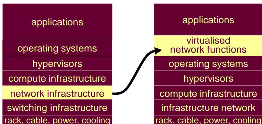
**Figure 6: Re-arrangement of the order of dependency between traditional application virtualisation (left) and network functions virtualisation (right)**
