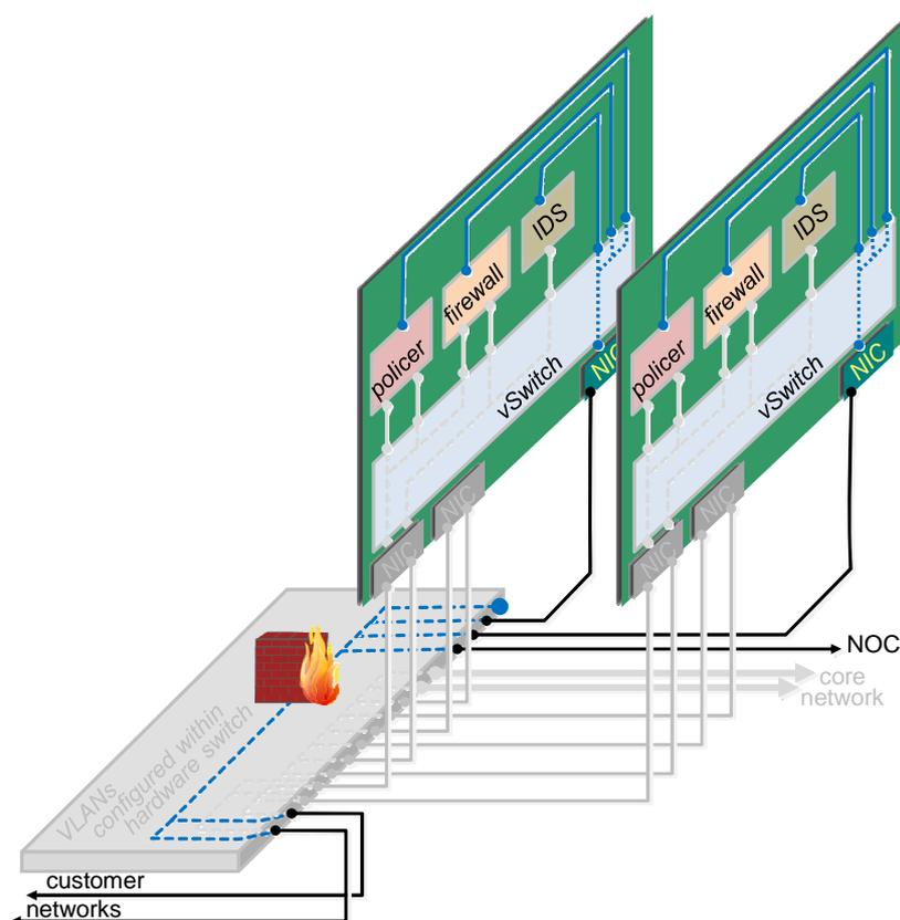
**Figure 7: Example management network, illustrating a mix of physical separation (core side) and logical separation (customer side and VNFs)**
