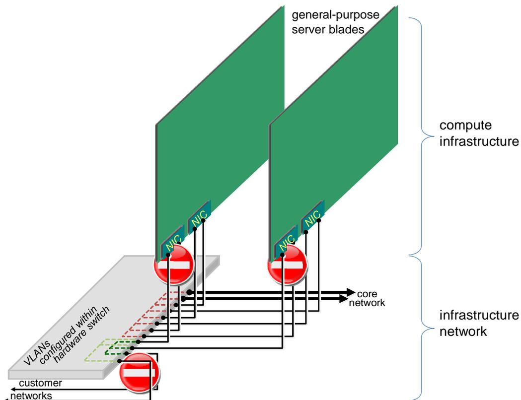
NOTE: The 'no entry' signs represent 'default-off' routing between partitioned infrastructure networks.
