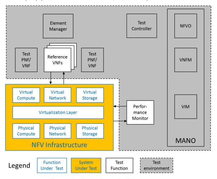
Figure 4.1: Functional architecture for NFVI under test
