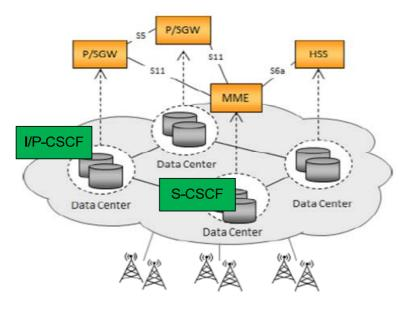
Figure A.6: An example of a virtualised EPC and IMS [i.5]
