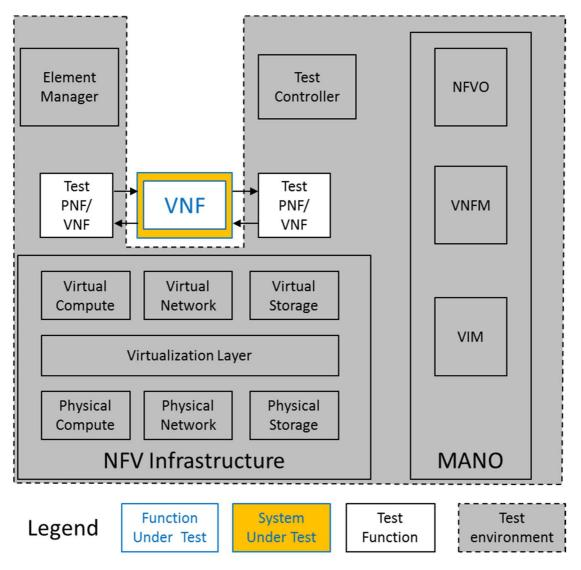
Figure 4.3: Functional architecture for VNF Under Test
