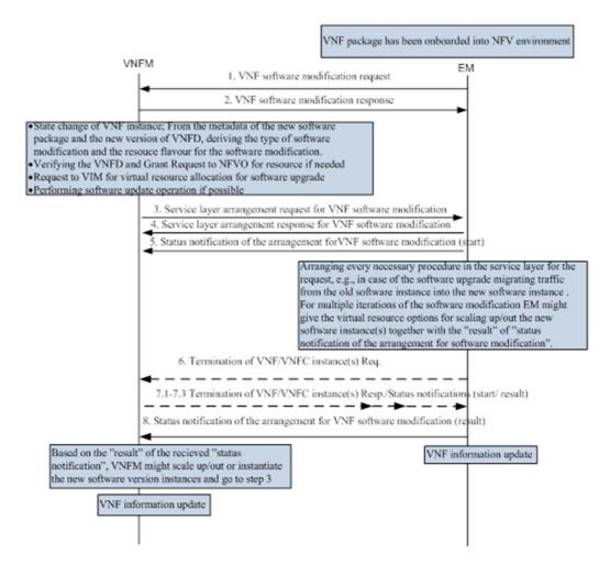
Figure B.2: Flow diagram for the operation of the VNF software modification initiated from EM
