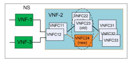
NOTE: Type 1 VNFC: VNFC11 and VNFC12 as redundancy pairs; Type 2 VNFC: VNFC22 and VNFC23 as a load sharing pool; Type3 VNFC: VNFC31, VNFC 32 and VNFC33 as another load sharing pool.
