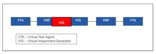
Figure 24: Fault injection using virtual impairment generator
