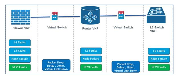
Figure 22: Challenge levels based on VNF type
