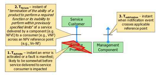
Figure 8: Canonical Failure Notification Model
