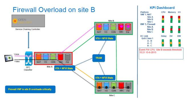
Figure 17: VNF Failure
