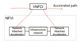
Figure 5.2-2: Accelerator chaining
