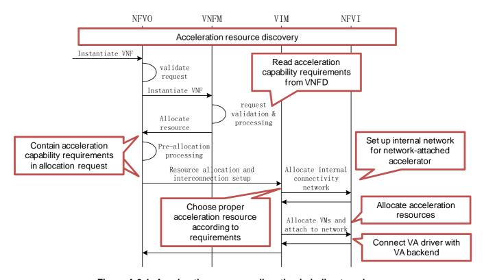
Figure A.2-1: Acceleration resource allocation in indirect mode
