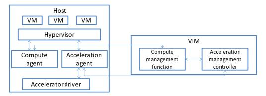
Figure B.2.1-1: Acceleration management architecture example
