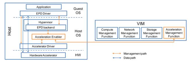
Figure 4.2.1-1: Acceleration resource management architecture
