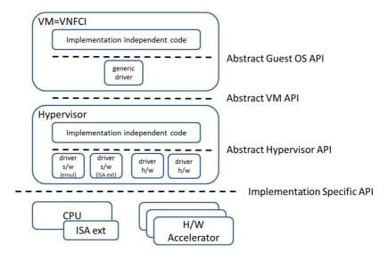
Figure 4.0-1: NFV acceleration abstraction layer implemented within hypervisor as a disaggregated model
