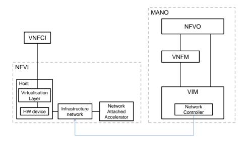
Figure 5.2-1: VNF and accelerator interconnection
