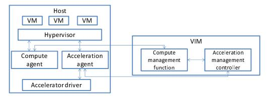
Figure B.2.1-1: Acceleration management architecture example
