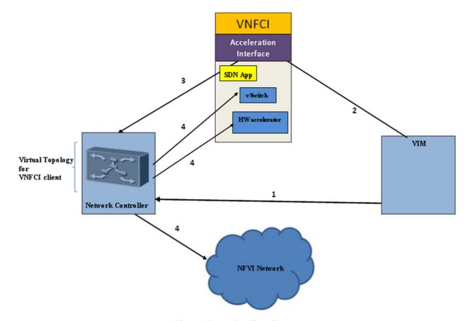
Figure 5.2-3: Traffic offload
