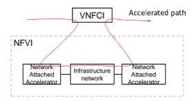
Figure 5.2-2: Accelerator chaining
