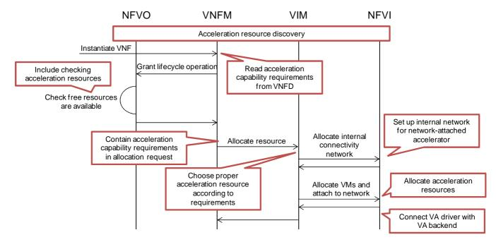
Figure A.2-2: Acceleration resource allocation in direct mode
