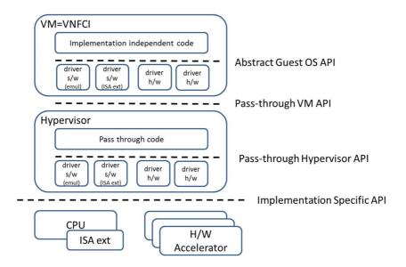
Figure 4.0-2: NFV acceleration abstraction layer implemented within VNF as an integrated model
