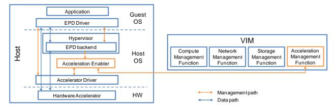
Figure 4.2.1-1: Acceleration resource management architecture
