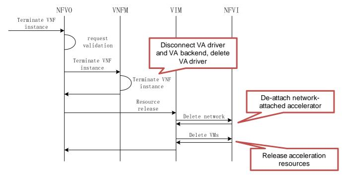
Figure A.3-1: Acceleration resource release in indirect mode
