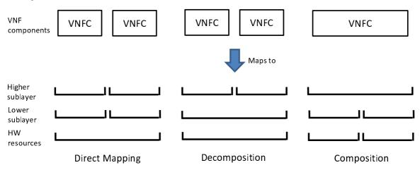
Figure 3: Virtualisation Container Interface Mapping
