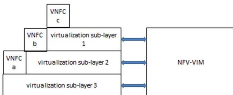
Figure 6: Example mixing of VNFCs on nested virtualisation technologies
