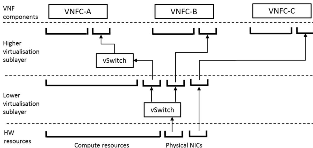
**Figure 4: Virtual Network Interface Mapping**
