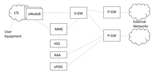
Figure 21: Typical elements of Evolved Packet Core within mobile network
