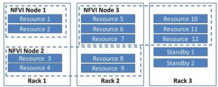
Figure 7: N:M NFVI Node to rack mapping
