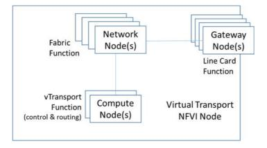
Figure 26: Virtual transport NFVI Node hardware decomposition showing network, gateway and compute nodes
