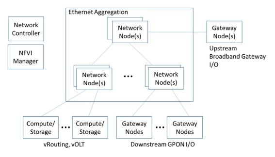
Figure 24: Architecture of access NFVI Node
