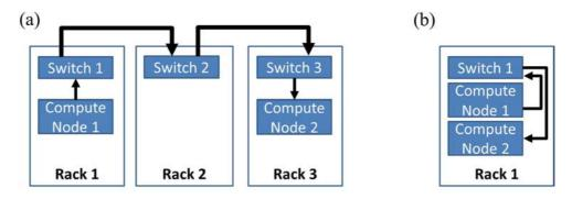
Figure 4: (a) geographically disperse compute nodes (b) compute nodes co-located within a single rack
