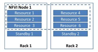
Figure 5: 1:N Mapping of NFVI Node to racks
