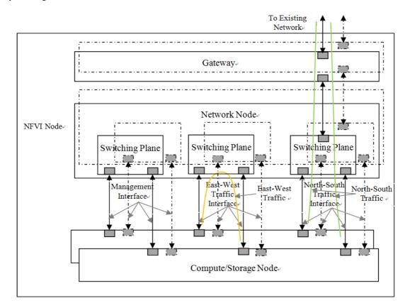
Figure 14: Example of physical interface and interconnection isolation in the NFVI Node
