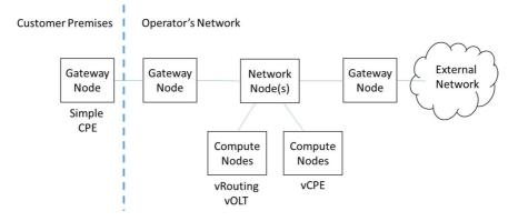
Figure 29: Virtual customer Premises Equipment using NFVI Node hardware
