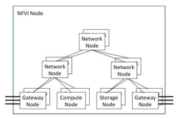
Figure 2: Example NFVI Node implementation including compute nodes and storage Nodes (equivalent to figure 22 of ETSI GS NFV-INF 003 [i.9])
