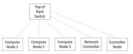
Figure 22: Hardware elements of virtual mobile network NFVI Node
