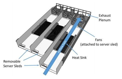
Figure 19: Simplified representative Open Compute servers showing cooling components and airflow path
