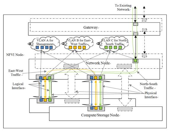
Figure 15: Example of logical interface and interconnection isolation in the NFVI Node
